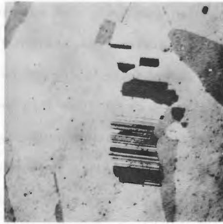
Fig. 2. Mg-reduced thorium as arc-melted. Polarized light. 200X.
