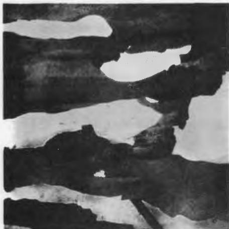
**Fig. 3. Mg-reduced thorium as arc-melted. Polarized light. 200X.**
