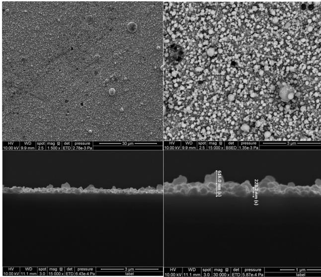
FIG. 1. (a) Secondary electron image at 1500 $\times$ , (b) BSE image at 15000 $\times$ , (c) cross section of thin film at 15000 $\times$ , and (d) thickness measurement on cross section at 30000 $\times$ .
