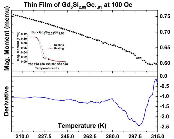
FIG. 2. (a)  $m$  vs.  $T$  at an applied field of at 100 Oe (7.9 kA/m). (b) Derivative of Fig. 2(a) showing the start and end of the phase transition. Inset figure shows the transition temperature of bulk sample of  $\text{Gd}_5\text{Si}_{2.09}\text{Ge}_{1.91}$ .
