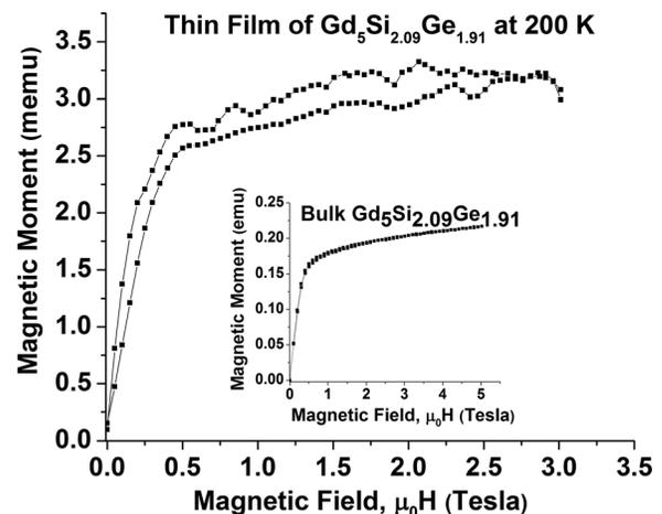
FIG. 3.  $m$  vs.  $\mu_0 H$  at 200 K showing the ferromagnetic nature of the material inset figure shows  $m$  vs.  $H$  measurement at 270 K on bulk sample of  $\text{Gd}_5\text{Si}_{2.09}\text{Ge}_{1.91}$ .
