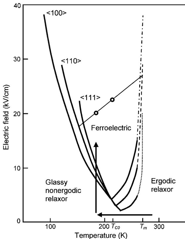
FIG. 9. The  $E$ - $T$  phase diagrams of  $\text{Pb}(\text{Mg}_{1/3}\text{Nb}_{2/3})\text{O}_3$  single crystals obtained from data presented in Figs. 6 and 7. The  $E_c(T)$  or  $T_{\text{ph}}(E)$  lines, delimiting the ferroelectric phase from the glassy nonergodic phase were attained from the measurement of ferroelectric hysteresis loops in different directions after zero-field cooling. The directions of the employed  $E$ - $T$  path are shown by thick arrows.
