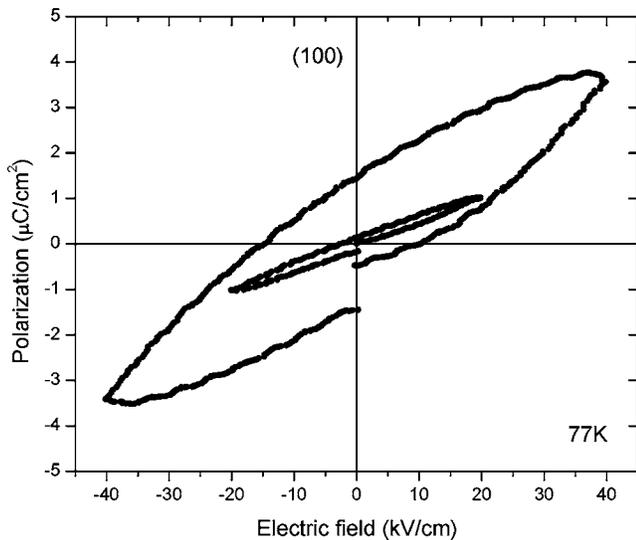
FIG. 8. Polarization vs electric field hysteresis loops measured at 4 Hz under  $\pm 20$  kV/cm and  $\pm 40$  kV/cm peak-to-peak fields in the (100)-oriented  $\text{Pb}(\text{Mg}_{1/3}\text{Nb}_{2/3})\text{O}_3$  crystal at 77 K.
