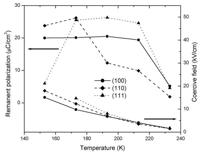
FIG. 6. Remanent polarization  $P_r$  and coercive field  $E_c$  as a function of temperature in the  $\text{Pb}(\text{Mg}_{1/3}\text{Nb}_{2/3})\text{O}_3$  single crystals. The  $E_c(T)$  lines will be replotted in Fig. 9 to delimit the ferroelectric phase from the glassy nonergodic relaxor phase.
