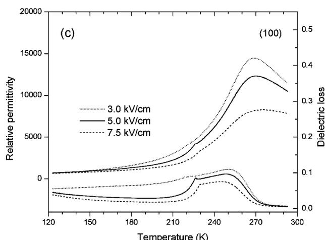
FIG. 3. Dielectric properties of  $\text{Pb}(\text{Mg}_{1/3}\text{Nb}_{2/3})\text{O}_3$  single crystals measured during field cooling at 1 kHz. (a) (111), (b) (110), and (c) (100) platelets.
