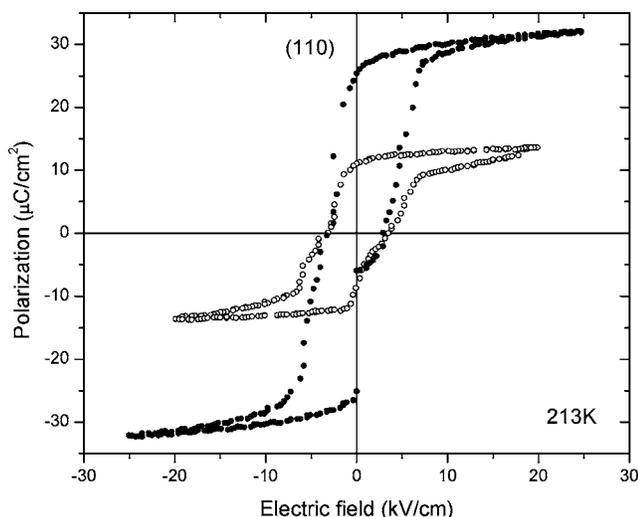
FIG. 10. Polarization vs electric field hysteresis loops measured at 4 Hz under  $\pm 20$  kV/cm and  $\pm 25$  kV/cm peak-to-peak fields in the (110)-oriented  $\text{Pb}(\text{Mg}_{1/3}\text{Nb}_{2/3})\text{O}_3$  crystal at 213 K.
