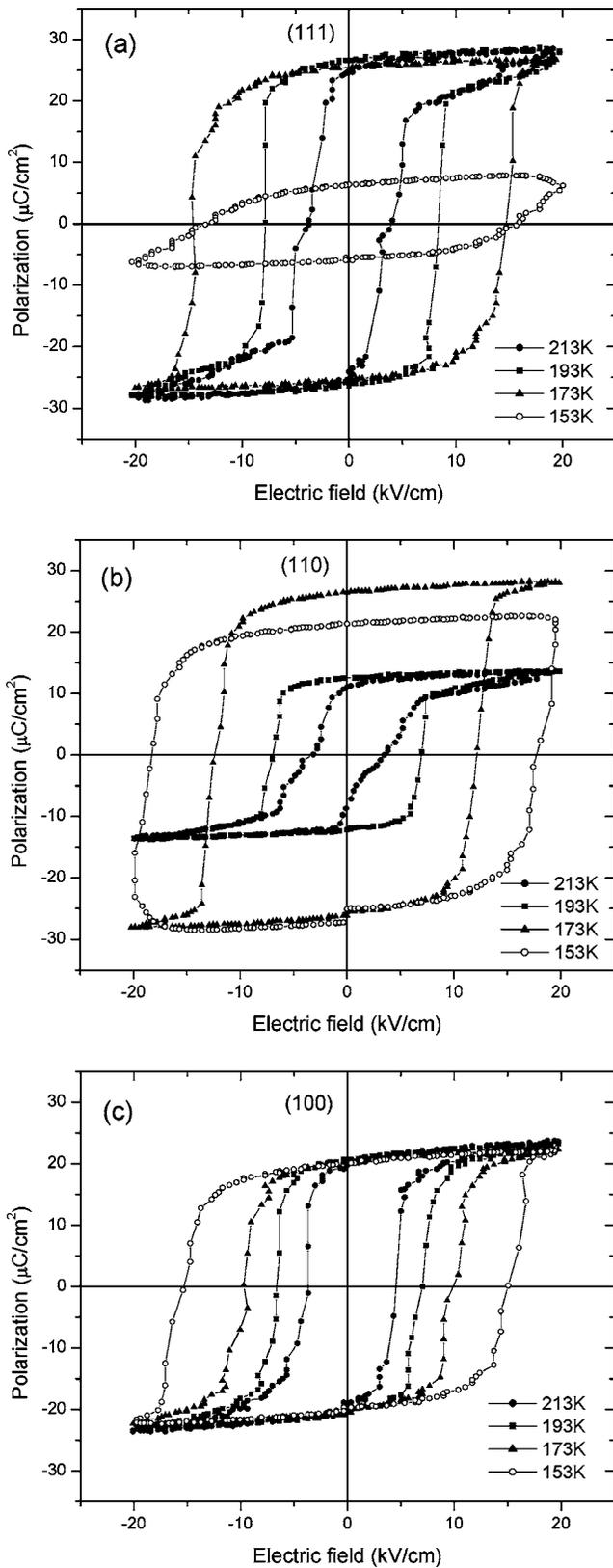
FIG. 5. Polarization vs electric field hysteresis loops measured at 4 Hz under a  $\pm 20$  kV/cm peak-to-peak field in  $\text{Pb}(\text{Mg}_{1/3}\text{Nb}_{2/3})\text{O}_3$  single crystals. (a) (111), (b) (110), and (c) (100) platelets.
