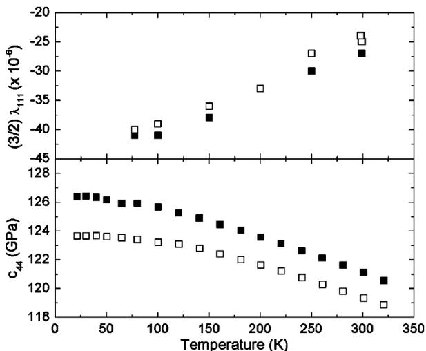
FIG. 2.  $(3/2)\lambda_{111}$  and elastic constant  $c_{44}$  as a function of temperature for  $\text{Fe}_{93.9}\text{Be}_{6.1}$  (■) and  $\text{Fe}_{88.7}\text{Be}_{11.3}$  (□) (Note the expanded scales).
