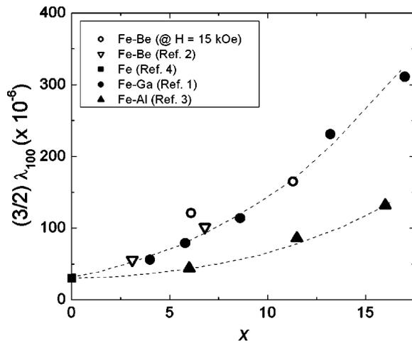
FIG. 4.  $(3/2)\lambda_{100}$  for  $\text{Fe}_{100-x}\text{X}_x$  ( $X=\text{Be, Ga, Al}$ ). Note the measured magnetostriction of  $\text{Fe}_{93.9}\text{Be}_{6.1}$  appears noticeably high and may reflect differences in composition between the measured sample and chemistry sample.
