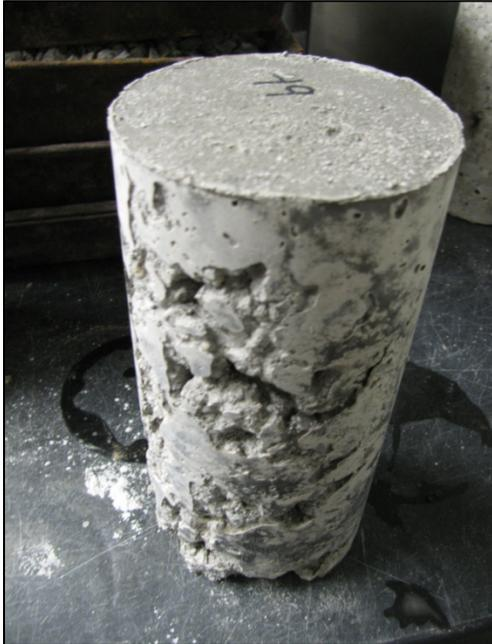
**FIGURE 12** Honeycombing occurred in the mixture containing 400 pcy cement content at a w/b of 0.65.
