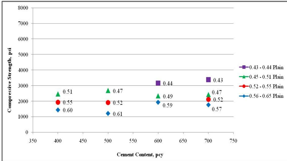
**FIGURE 7** Effect of different w/b with various levels of cement content on 1 day compressive strength.
