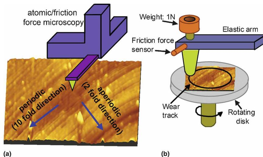
FIG. 1. Schematic illustration of the friction measurement on oxidized Al–Ni–Co decagonal quasicrystal surface: (a) friction/atomic force microscopy experiment and (b) pin-on-disk experiment. (color online)
