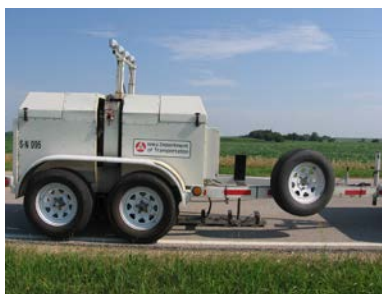
Figure 1. Falling Weight Deflectometer (FWD) Equipment Used for Non-Destructive Testing of Pavements
