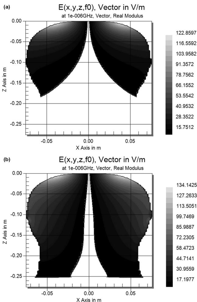
FIG. 3. Contour plots of electric field distribution in central coronal slice of (a) circular 90 mm coil alone and (b) with Halo coil.
