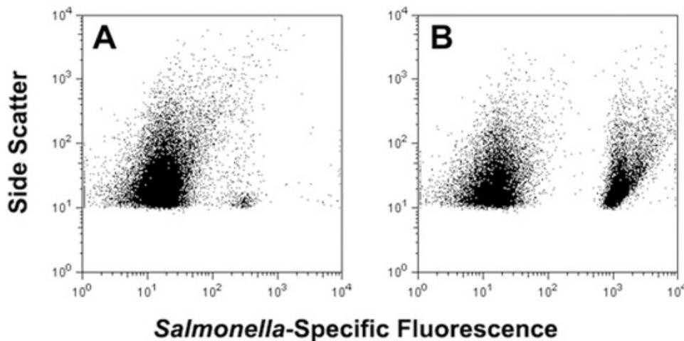
**Figure 4.** Use of adhesive tape for sampling of *S. enterica* serovar Typhimurium from the surface of an artificially contaminated tomato, followed by direct analysis via FISH and flow cytometry (panel A) or after 5 h non-selective liquid surface miniculture enrichment in a perfusion chamber filled with 500  $\mu$ L Trypticase Soy Broth (panel B).
