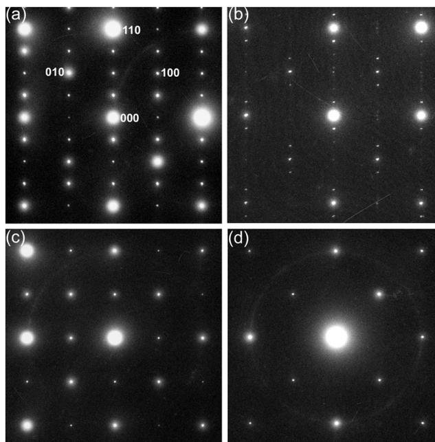
FIG. 4. Hot stage *in situ* TEM experiment on a thin foil specimen of the PZ98-PNN2 ceramic. The  $\langle 001 \rangle_c$ -zone axis SAED patterns observed during heating at (a)  $25^\circ\text{C}$ , (b)  $179^\circ\text{C}$ , (c)  $194^\circ\text{C}$ , and (d)  $240^\circ\text{C}$ .
