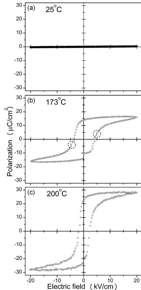
FIG. 3. Polarization hysteresis loops recorded from a bulk PZ98-PNN2 ceramic at 4 Hz during heating at (a)  $25\text{ }^{\circ}\text{C}$ , (b)  $173\text{ }^{\circ}\text{C}$ , and (c)  $200\text{ }^{\circ}\text{C}$ .
