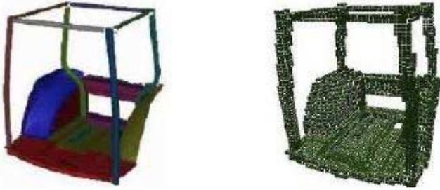
Figure 3: Comparison of the exact model with the voxelized approximation
