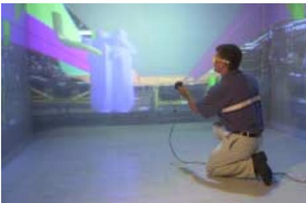
Figure 7: Assembling a parking brake component under the cab in the VEGAS environment
