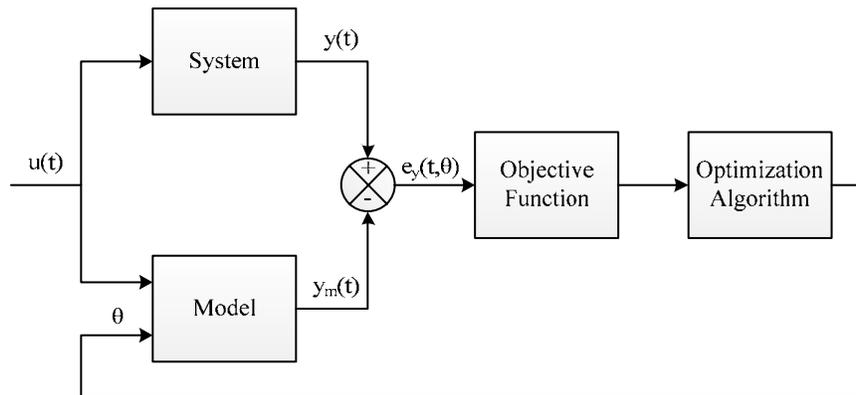
Figure 2 - The general parameter identification process (adapted from similar figures given by Walter and Pronzato (1997))
