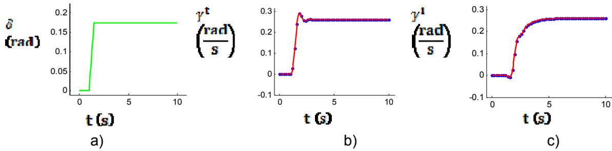
Figure 3 - Time histories of a) front wheel steering input (rad) and simulated data with signal-to-noise ratio of 1000 for b) tractor yaw rate (rad/s), and c) implement yaw rate (rad/s).
