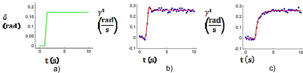
Figure 5 - Time histories of a) front wheel steering input (rad) and simulated data with signal-to-noise ratio of 25 for b) tractor yaw rate (rad/s), and c) implement yaw rate (rad/s).
