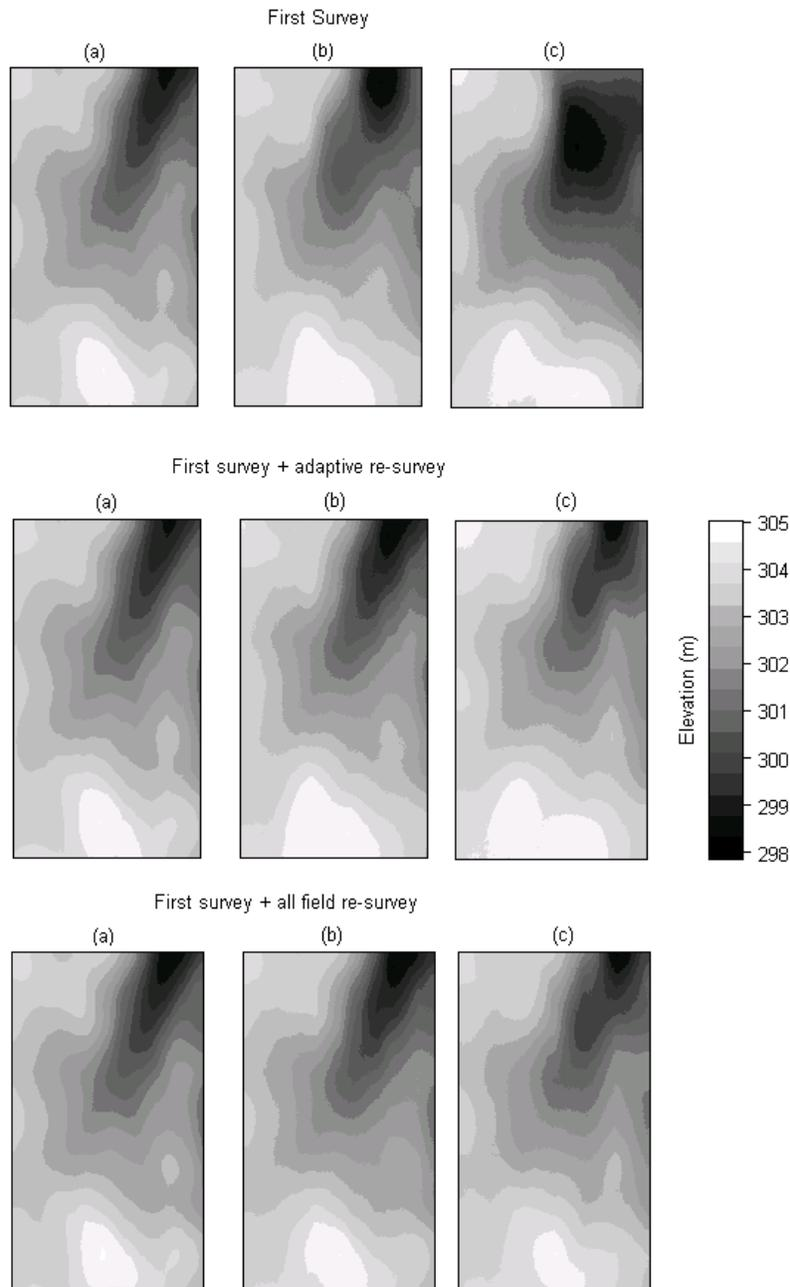
Figure 9. Contour plots of DEMs using measurements at (a) 6.10 m, (b) 15.25 m, and (c) 24.40 m pass intervals.
