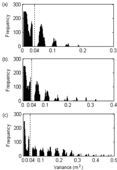
**Figure 3.** Histograms of SGS variance estimates using measurement passes at (a) 6.10 m, (b) 15.25 m, and (c) 24.40 m intervals. The dashed vertical line is the variance threshold above which grids were classified as highly uncertain regions.
