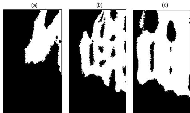
**Figure 4.** Conditional variance maps for measurements at (a) 6.10 m, (b) 15.25 m, and (c) 24.40 m pass intervals were transformed into binary images. Low-uncertainty regions (white) were classified by image segmentation with the 0.4 m<sup>2</sup> threshold followed by the morphological operation functions of “cleaning,” “filling,” and “removing” implemented in Matlab.
