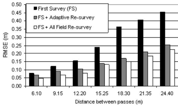
Figure 7. RMSE of DEMs developed using measurements across different passes intervals and with additional adaptive and all-field re-survey measurements between the passes.
