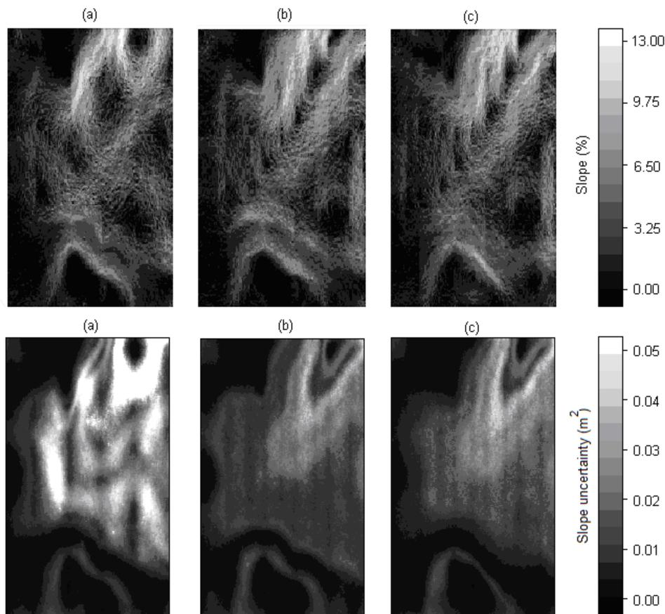
Figure 10. (a) Plots of slope using measurements at 15.25 m pass intervals (top) and associated uncertainty maps (bottom). Additional adaptive and all-field re-survey measurements were added to generate maps in (b) and (c), respectively.
