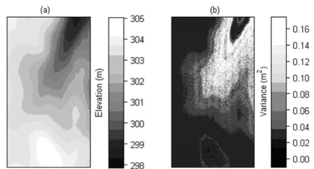
Figure 2. (a) Mean elevation (E-type) estimate and (b) corresponding conditional variance map of the DEM generated from SGS using measurements with 6.10 m pass intervals.
