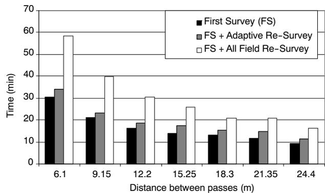
**Figure 6.** Estimated time to collect the elevation data with additional adaptive and all-field re-survey measurements as a function of distance between passes.
