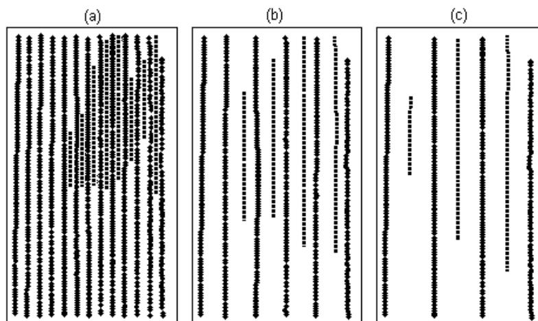
Figure 1. Measurements passes at (a) 6.10 m, (b) 15.25 m, and (c) 24.40 m intervals (diamonds) with additional adaptive re-survey measurements between the passes (squares).
