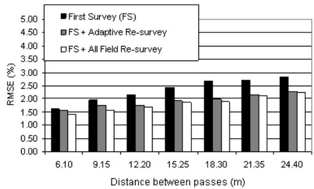
Figure 8. RMSE of slope derived from DEMs developed using measurements across different passes interval and with additional adaptive and all-field re-survey measurements between the passes.
