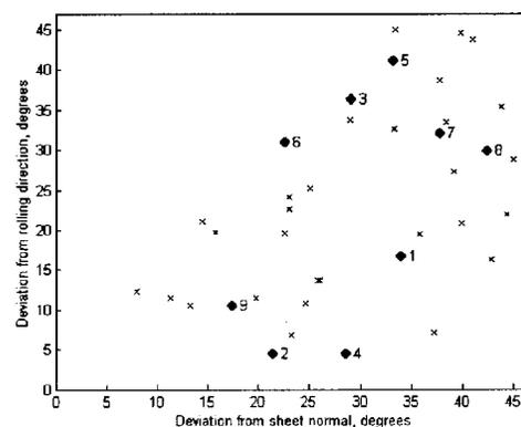
FIG. 2. Angular deviations of grains' crystallographic orientation from a  $\{001\}\langle 100\rangle$  sheet texture in 1100 °C annealed rolled  $\text{Fe}_{83}\text{Ga}_{17}$ . Numbered data points (●) correspond to grains in the strain gauged area of Fig. 1. The data points indicated by  $\times$  represent adjacent mapped grains.
