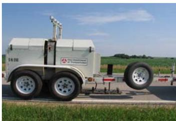
Figure 1. Picture of Iowa DOT's JILS-20 FWD equipment.
