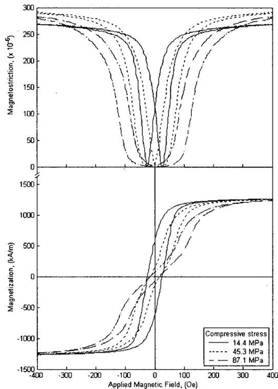
FIG. 1. Applied magnetic field dependencies of the magnetostriction and magnetization of  $\text{Fe}_{0.81}\text{Ga}_{0.19}$  at  $80^\circ\text{C}$  for various compressive stresses. All measurements were made at 0.05 Hz in a flux-closed transducer.
