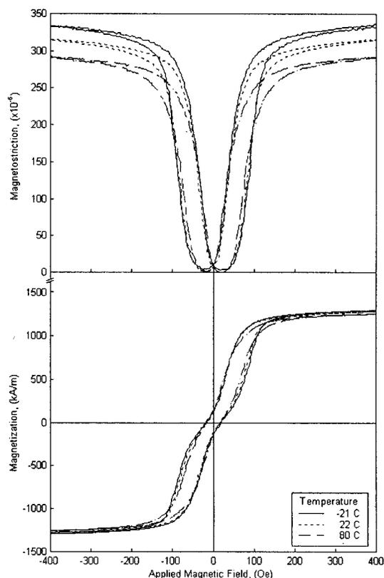
FIG. 3. Applied magnetic field dependencies of the magnetostriction and magnetization of  $\text{Fe}_{0.81}\text{Ga}_{0.19}$  at 45.3 MPa for three temperatures.
