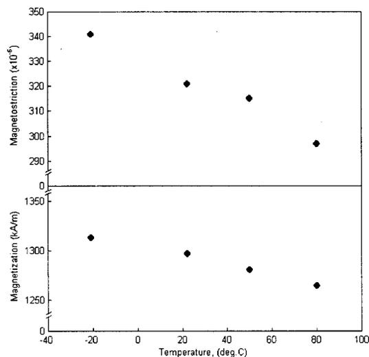
FIG. 4. Temperature dependencies of the maximum magnetostriction and magnetization of  $\text{Fe}_{0.81}\text{Ga}_{0.19}$  for a 45.3 MPa compressive stress and 800 Oe applied field.
