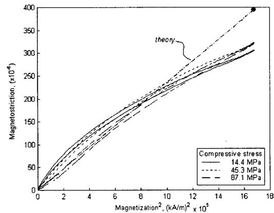
FIG. 2. Magnetization squared dependencies of the magnetostriction of  $\text{Fe}_{0.81}\text{Ga}_{0.19}$  at  $22^\circ\text{C}$  for three compressive stresses.
