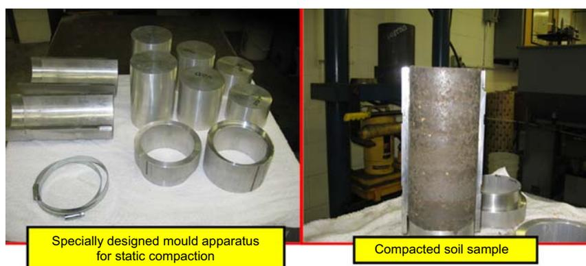
**Figure 4.** Subgrade soil sample preparation for resilient modulus test
