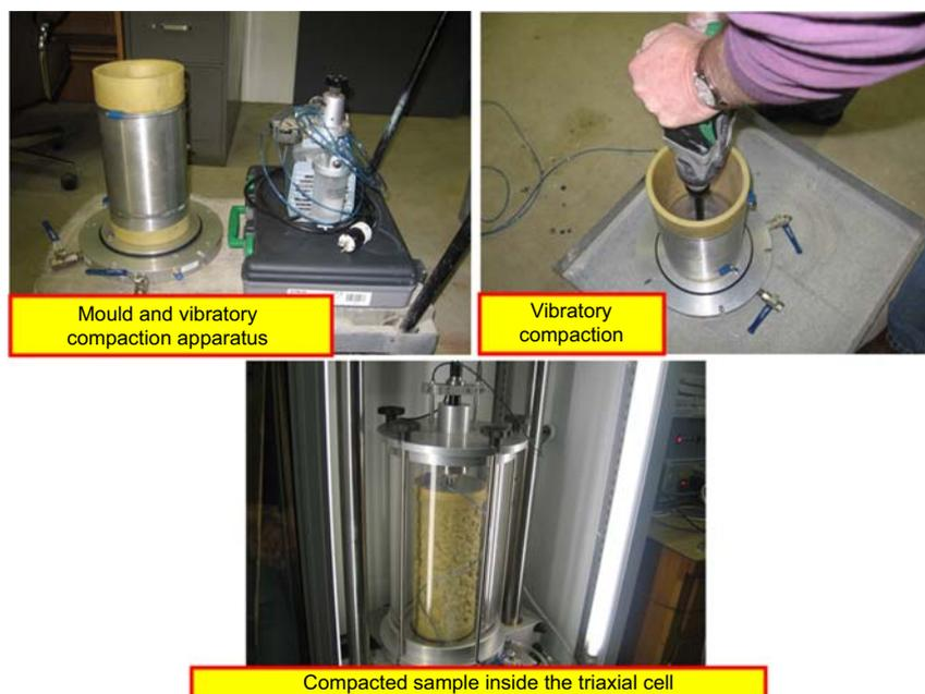
Figure 5. Base/sub-base aggregate sample preparation for resilient modulus test
