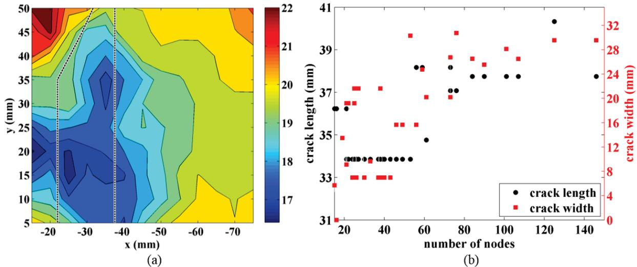
**Figure 6. (a) Wavelet resolution map showing the average wavelet bandwidths for a representation using 59 nodes (the approximate crack region is shown within the black-dashed region); and (b) Identified crack length and width based on wavelet resolutions.**
