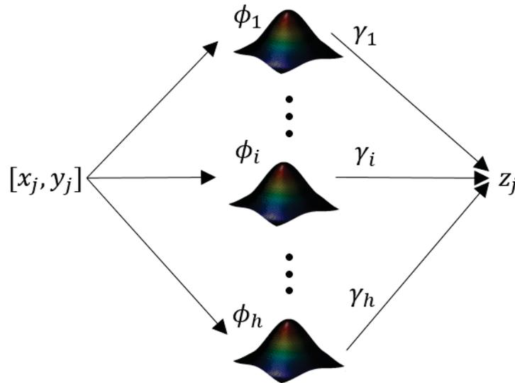
**Figure 2. Single-layer architecture of the wavelet network**
