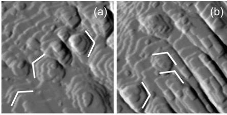
FIG. 11. [(a) and (b)] STM images of a Ag film, about 40 layers thick, on NiAl(110) at 200 K. Several sets of  $120^\circ$  angles are illustrated with the white lines. The images have been differentiated to accentuate the step edges. Each image size is  $100 \times 100 \text{ nm}^2$ .
