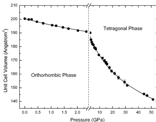
FIG. 7. The change of AgN<sub>3</sub> unit cell volume with pressure. The solid lines demonstrate the fitting of the P-V data to the third-order Birch-Murnaghan equation of state.
