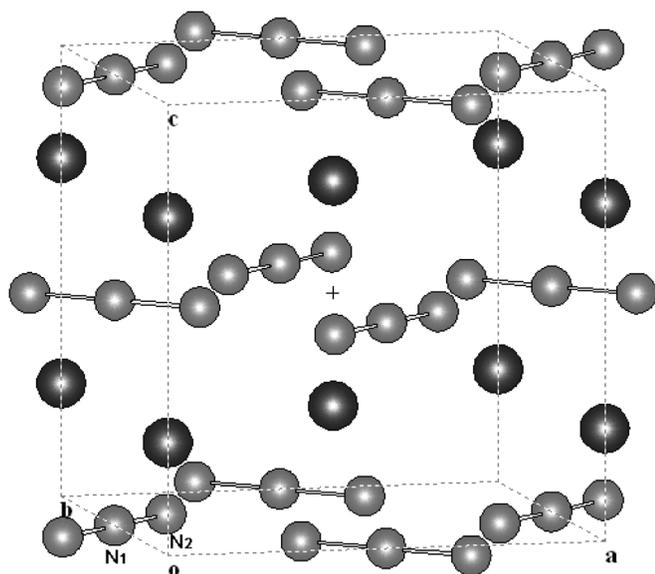
FIG. 6. The crystal structure of HP-AgN<sub>3</sub> yielded from the refinement at 13.8 GPa. The Ag atoms are represented by black spheres and N atoms by gray spheres.
