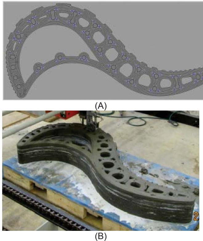
**Figure 2 – Complex Concrete Printing Product (a) 3D Model (Lim et al. 2012), (b) During printing (Le et al. 2012)**
