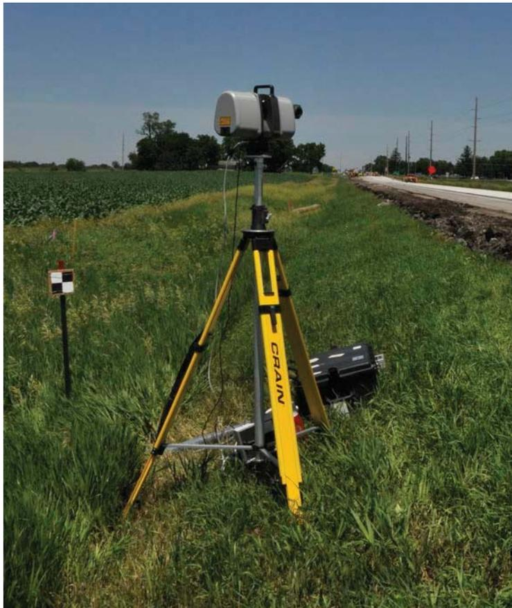
**Figure 1. Trimble CX 3D laser scanner set-up.**
