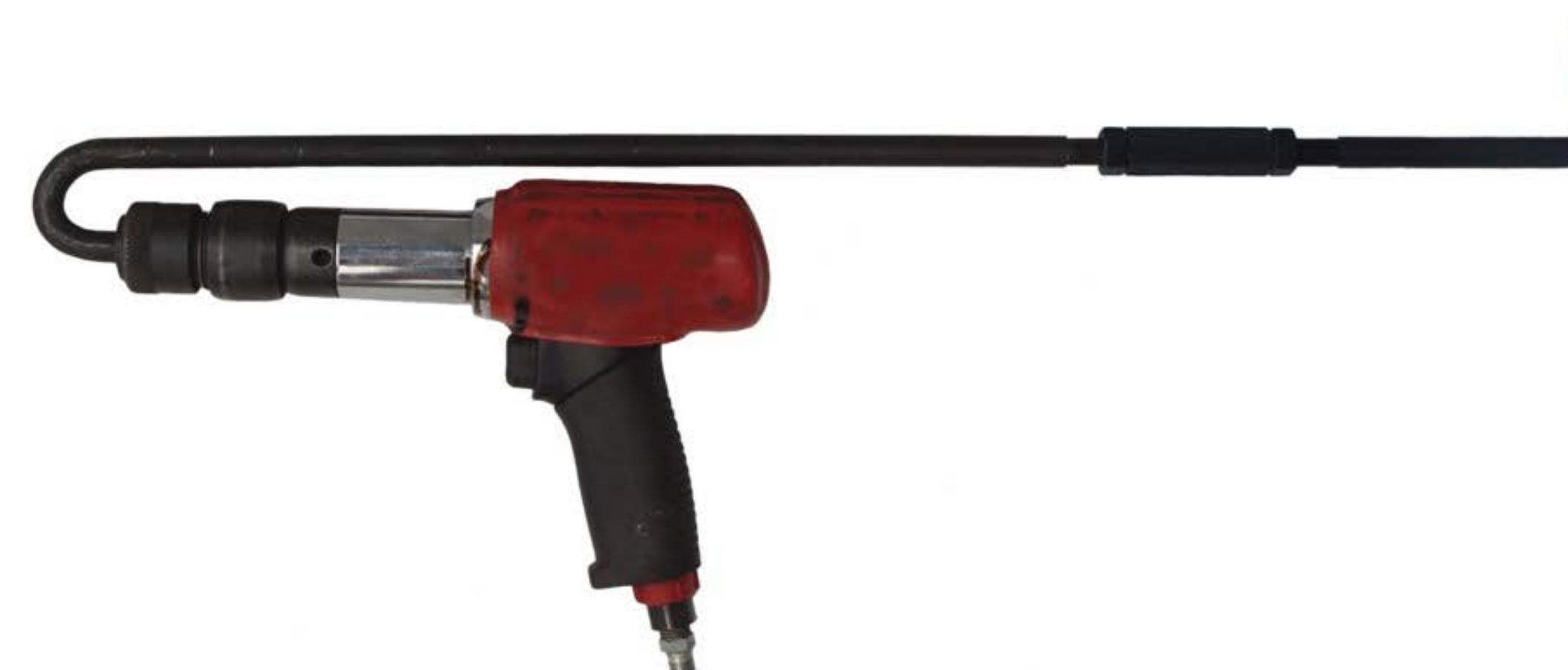
Right: The "Texas Twister" air hammer puller adapter installed on a pneumatic air hammer. Photo credit: vehicleservicepros.com
