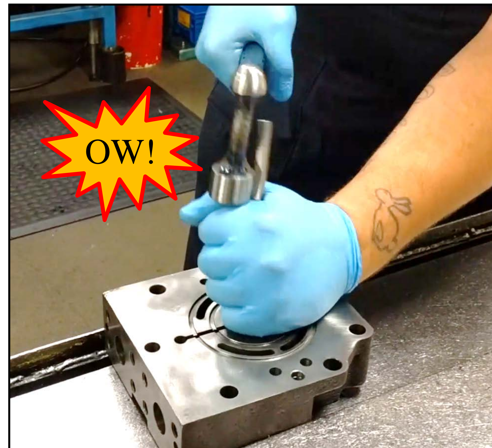
Left: Technician strikes hand with hammer while chiseling a bearing from a casting. Above: mangled bearing introduces metallic contamination to clean assembly area. Photo credit Ben Gibson
