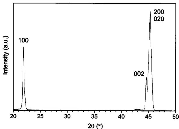
FIG. 2. X-ray diffraction indicates a  $\{010\}$  surface plane, a tetragonal symmetry, and a high volume fraction of  $a$  domains with in-plane polarization.
