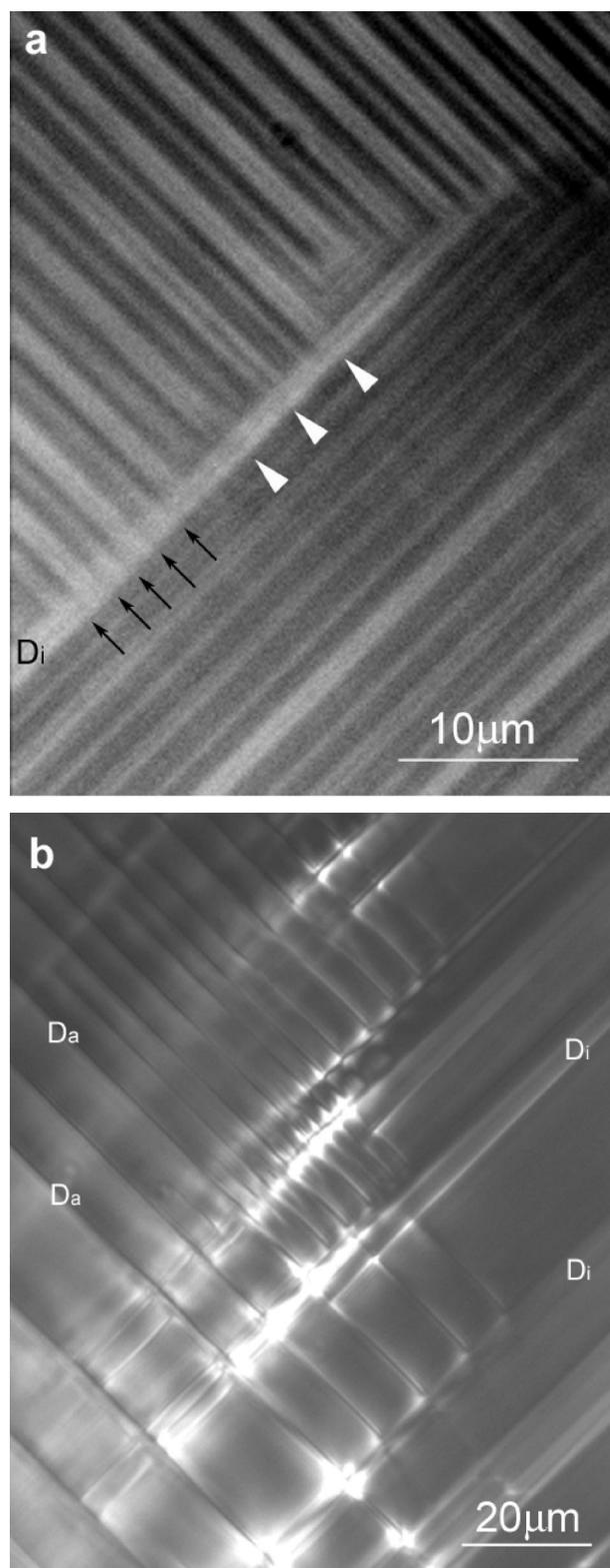
FIG. 5. Domain configurations near the zone boundary. (a) Full contact of orthogonal  $90^\circ$  domain strips is indicated by bright triangles. The faint contrast in the impinging domain  $D_i$ , pointed out by dark arrows, suggests the domains have grown into the  $D_i$ . (b) Interpenetration of orthogonal  $90^\circ$  domain strips. The approaching domains  $D_a$  penetrate the impinging domains  $D_i$  and short segments of  $D_i$  are formed.
