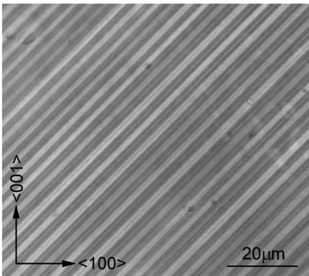
FIG. 1. Initial domain structure in the annealed specimen of 0.65PMN–0.35PT crystal.
