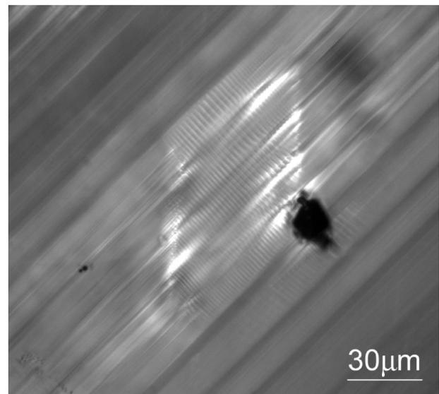
FIG. 7. Nucleation of a domain zone with orthogonal domain strips around an inclusion in an as-grown PMN-PT crystal.
