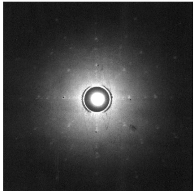
FIG. 3. X-ray Laue diffraction pattern used to determine the in-plane orientations.
