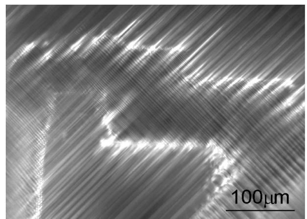
FIG. 4. Development of domain zones of  $90^\circ$  domain strips orthogonal to the preexisting domain strips after bipolar electric fields for 36 000 cycles at  $\pm 4.0$  kV/cm and 36 000 cycles at  $\pm 5.0$  kV/cm.
