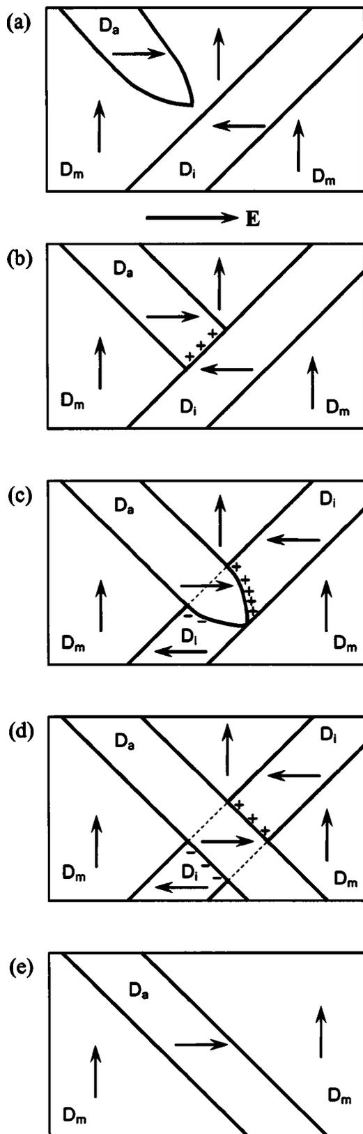
FIG. 6. Domain configurations at different stages of evolution. (a) Initial domain structure; (b) the full contact of two intersecting domains; (c) advance of the approach domain by the 180° domain switching; (d) the outgrowth step; and (e) the final withdrawal step.
