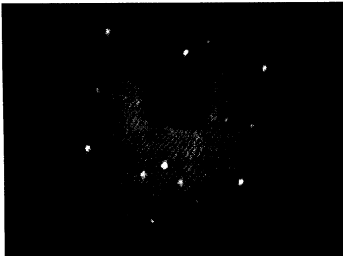
Figure 4. LEED pattern at 100 eV incident electron energy and normal incidence after annealing at 900 K for 2 hours.
