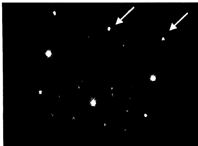
Figure 2a. LEED pattern at 60 eV incident electron energy and normal incidence after annealing at 800 K for 2 hours. The left and right arrows denote the (0,1) and (1,1) spots, respectively.
