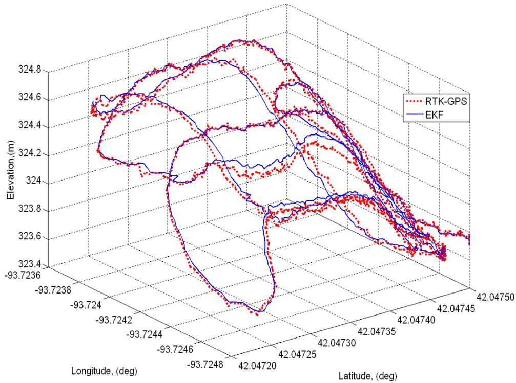
Figure 7: Sprayer travel trajectory (3D) measured by RTK-GPS and estimated by EKF data fusion technique.
