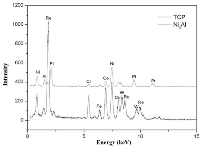
FIG. 2. EDX spectra of the  $\mu$  and  $\gamma'$  phases in the coating.
