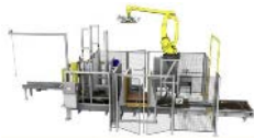
Robotic palletizing system
