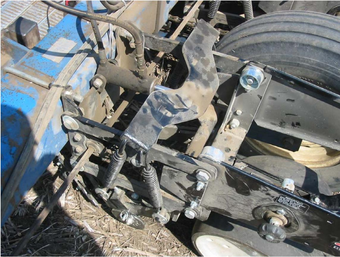
**Figure 2. Down-pressure adjustment mechanism to change spring length on parallel links (seed hopper normally to right removed for clarity).**
