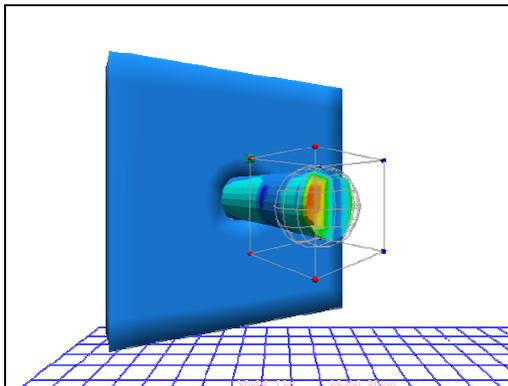
**Figure 8: Pin and base assembly with reduced Von Mises Stress.**
