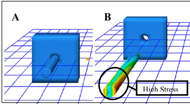
**Figure 7: A: pin and base assembly, B: base assembly with Von Mises Stress in IVDA.**
