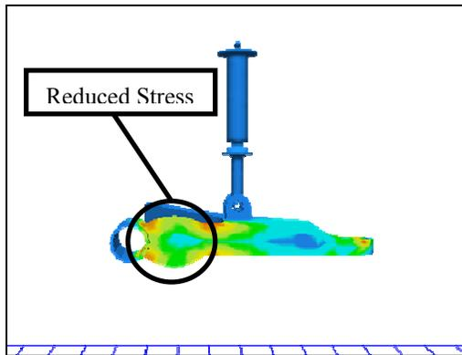
**Figure 10: New geometry of control arm while assembled with suspension.**
