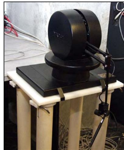
**Figure 5: PHANTOM haptic device**
