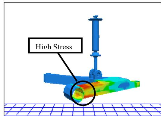
**Figure 9: Suspension assembly in the IVDA with stresses.**
