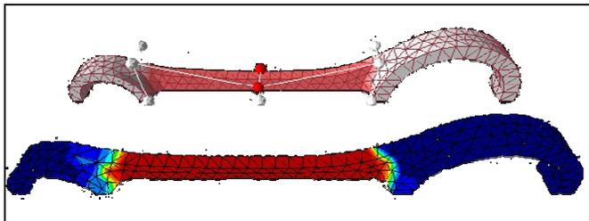
Figure 2: Deformed connecting rod with Taylor series stress approximations [5].
