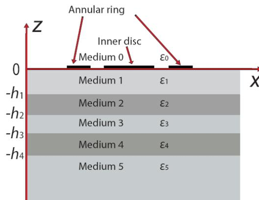
**FIGURE 2.** Concentric capacitive sensor on top of a five-layer dielectric.
