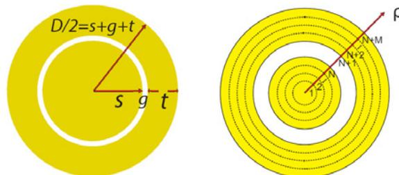
**FIGURE 1.** Concentric coplanar capacitive sensor. The radius of the central disc and the width of the outer ring are  $s$  and  $t$ , and the gap in between is  $g$ . For computational purposes, the sensor is divided into  $N$  circular filaments on the inner disc and  $M$  circular filaments on the outer annular ring.
