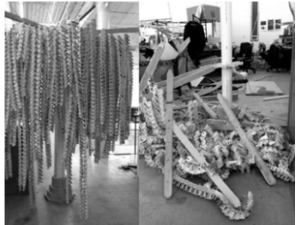
Fig. 3. Prototype pre-, and post-collapse.
