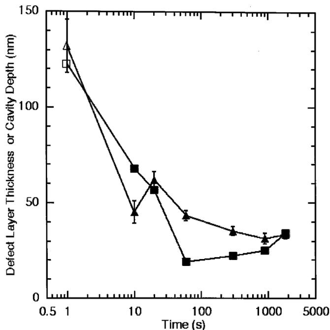
**Figure 11.** Comparison of model defect layer thickness (from Fig. 5) and mean cavity depth from AFM images of foils treated in NaOH followed by stripping oxide film in chromic-phosphoric acid. Error bars denote 90% confidence intervals based on measurement of between 25 and 50 cavities.
