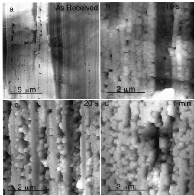
**Figure 9.** Top view AFM images after dissolution of foils in 1 M NaOH for various times, followed by oxide film stripping in chromic-phosphoric acid bath. (a) As-received, stripping time 1.5 min, height contrast 440 nm; (b) 10 s in NaOH, stripping time 2.5 min, 151 nm; (c) 20 s in NaOH, stripping time 1.5 min, 270 nm; (d) 1 min in NaOH, stripping time 1.5 min, 270 nm.
