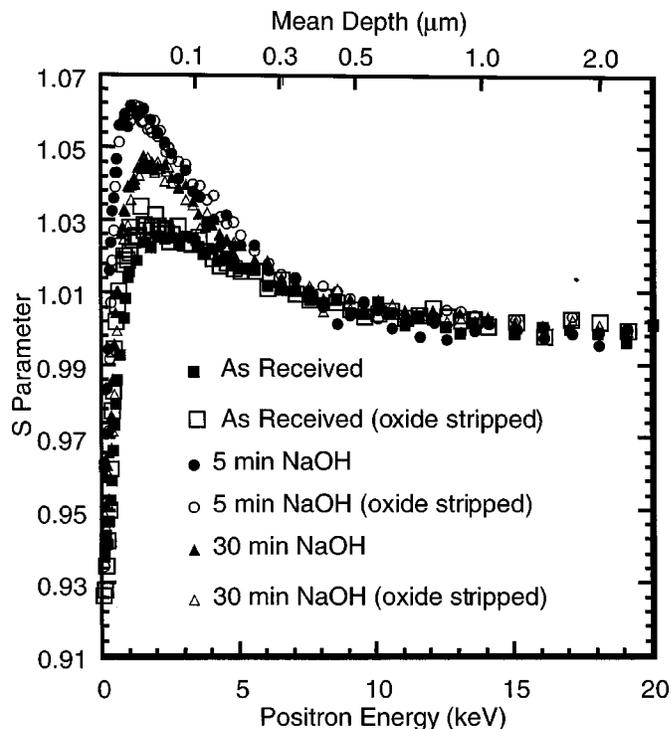
**Figure 13.** Effect of chromic-phosphoric acid oxide stripping treatment on  $S$  energy profiles. Open and closed symbols are for foils before and after oxide stripping treatment. Immersion times in stripping bath are as-received, 1.5 min; 5 min NaOH, 1 min; 30 min NaOH, 1 min.
