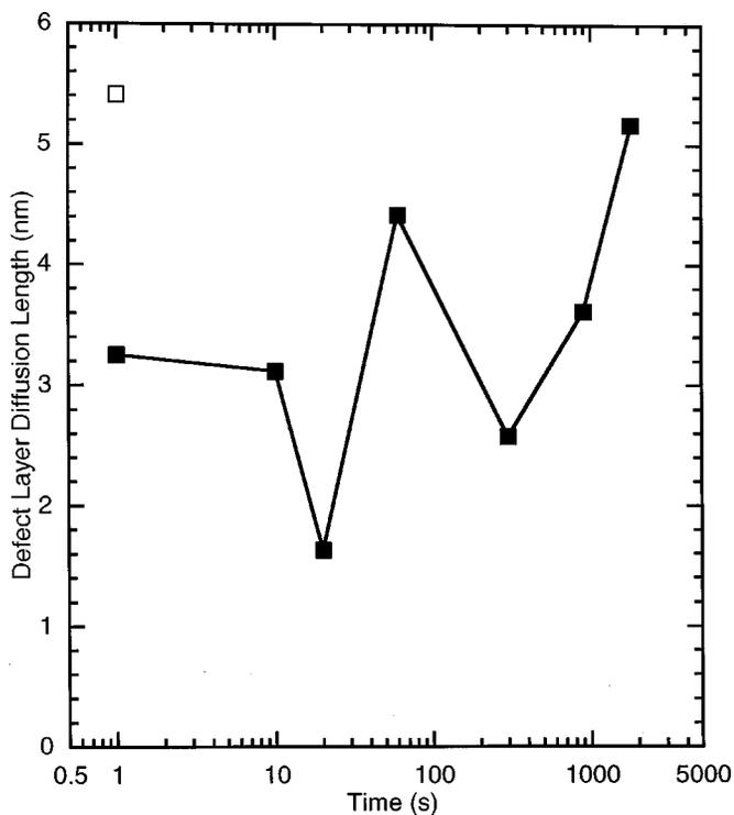
**Figure 6.** Model defect layer positron diffusion length vs. dissolution time. Open square is for as-received foil.
