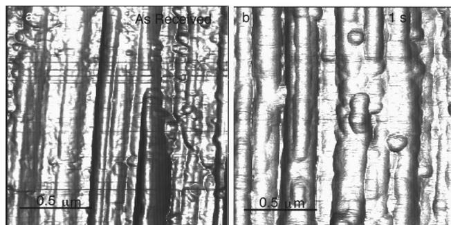
**Figure 8.** Illuminate view images comparing foil surface (a) as-received and (b) after 1 s dissolution.
