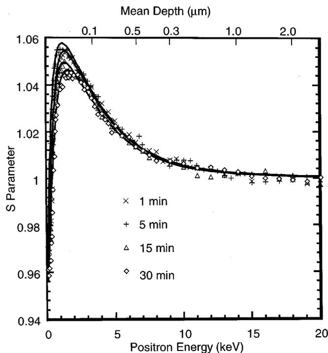
**Figure 2.**  $S$  energy profiles of foils after dissolution for 1, 5, 15, and 30 min. Data points are measured values, and solid lines are results of fitting with the simulation. Top scale is mean implantation size from Eq. 1.
