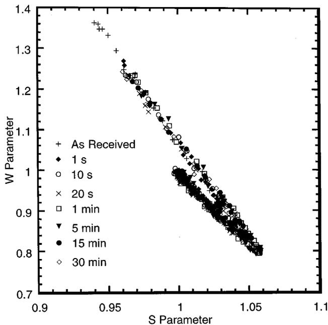
**Figure 3.** Plot of experimental  $W$  and  $S$  parameters for as-received foil and for all dissolution times.  $W$  and  $S$  are normalized with respect to their values for the bulk metal.
