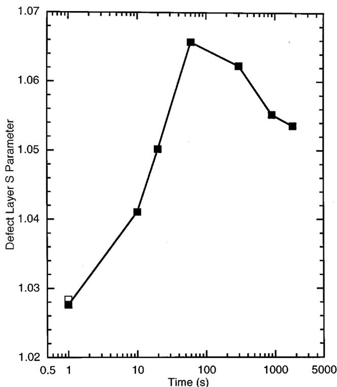
**Figure 4.** Model defect layer  $S$  parameter vs. dissolution time. Open square is for as-received foil.
