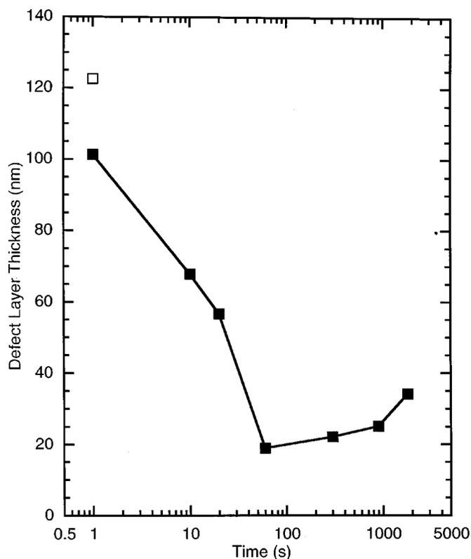
**Figure 5.** Model defect layer thickness fit vs. dissolution time. Open square is for as-received foil.
