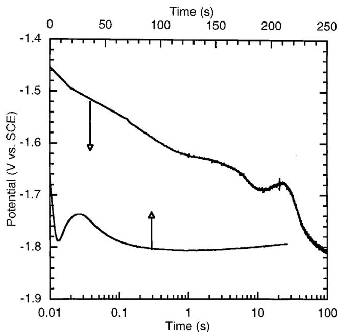
**Figure 15.** Potential transients during dissolution plotted to demonstrate both early- and long-time behavior.
