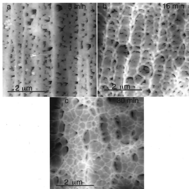
**Figure 10.** Top view AFM images after dissolution of foils in 1 M NaOH for various times, followed by oxide film stripping time for 1 min in chromic-phosphoric acid bath. (a) 5 min in NaOH, height contrast 162 nm; (b) 15 min in NaOH, 100 nm; (c) 30 min in NaOH, 176 nm.
