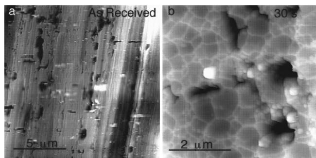
**Figure 14.** AFM images of foils etched in mixed 1 M HCl-6 M H<sub>2</sub>SO<sub>4</sub> bath at 90°C for 5 s, at applied current density of 0.3 A/cm<sup>2</sup>. (a) As-received foil used for etching, height contrast 440 nm. (b) Foil pretreated by 1 M NaOH immersion for 30 min, 500 nm.
