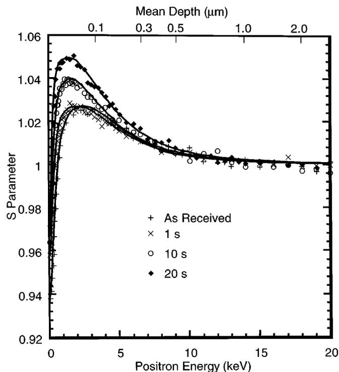
**Figure 1.**  $S$  energy profiles of as-received aluminum foil, and after dissolution in NaOH for 1, 10, and 20 s. Data points are measured values, and solid lines are results of fitting with simulation. Top scale is mean implantation depth according to Eq. 1.
