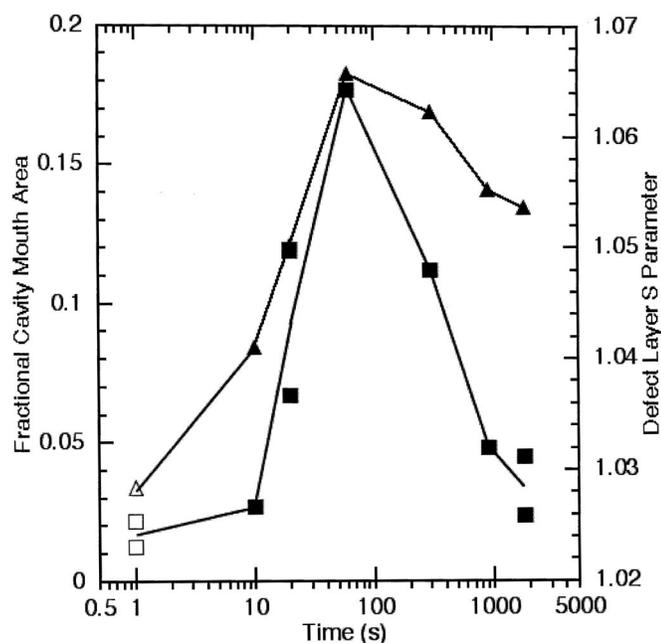
**Figure 12.** Comparison of model defect layer  $S$  parameter (from Fig. 4) and the fractional coverage of the foil surface with cavities, the latter estimated using AFM image analysis.
