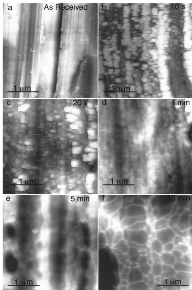
**Figure 7.** Top view AFM images after dissolution of foils in 1 M NaOH for various times: (a) as-received, height contrast 90 nm; (b) dissolution time 10 s, height contrast 80 nm; (c) 20 s, 111 nm; (d) 1 min, 85 nm; (e) 5 min, 80 nm; (f) 15 min, 105 nm.
