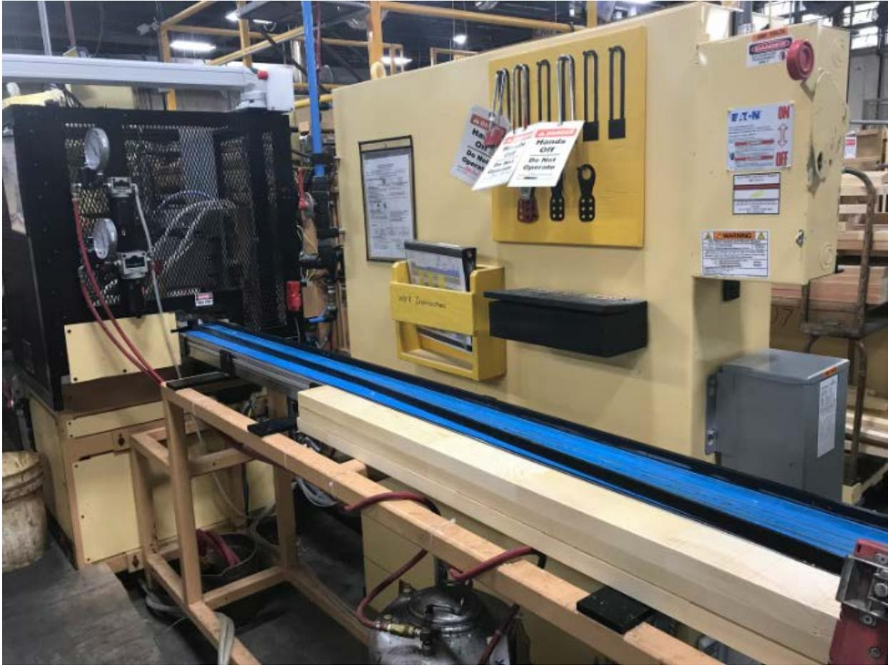
Figure 2.6 Edgeband fixture preload to press
