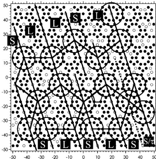
FIG. 4. Atomic positions in a plane ( $10 \times 10 \text{ nm}^2$ ) generated from experimental bulk structure model. Filled circles: Al atoms. Unfilled circles: Fe atoms. The sketched contour illustrates the matching part of the STM image outlined in Fig. 3.
