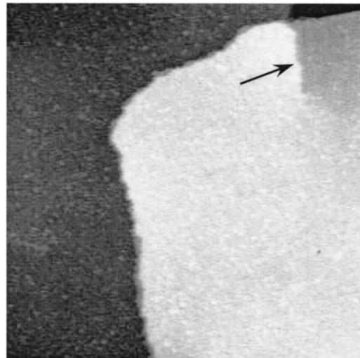
FIG. 1. STM image ( $100 \times 100 \text{ nm}^2$ ) showing the typical step-terrace structure. The arrow indicates a screw dislocation; these are often observed on the *5f* *i*-Al-Cu-Fe surface.<sup>4</sup>
