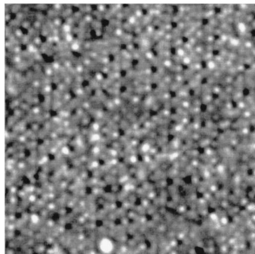
FIG. 5. High resolution STM image ( $20 \times 20 \text{ nm}^2$ ) of an *i*-Al-Pd-Mn  $5f$  surface, obtained under experimental conditions very similar to those of Figs. 2 and 3, and with the same experimental apparatus.
