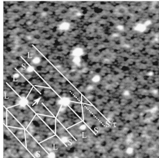
FIG. 3. Same high resolution STM image as in Fig. 2. Pentagons are drawn to illustrate the local  $5f$  arrangements of flowers. Parallel lines separated by different spacings align the flowers. The arrow indicates where a displacement takes place. The splitting of a wider spacing into two smaller ones is shown in the upper-right-most spacing.
