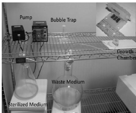
**FIGURE 1.** Set-up of the flow system for biofilm growth
