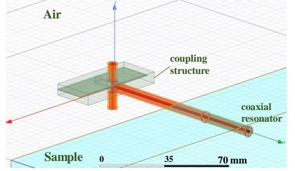
Fig. 3 Resonant sensor model on HFSS
