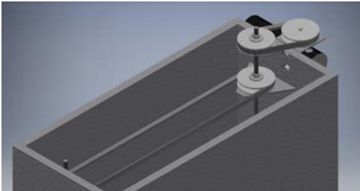
*Figure 2. Proposed Solution 2: belt and pulleys. This design was not chosen because of the high chance of the belts slipping and being inefficient in transmitting power. Belts also become brittle over time.*
