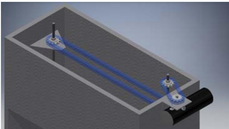
Figure 3. Proposed Solution 3: sprockets and chain. This solution was the most cost-effective way of transferring power from the motor to the shafts. The low amount of moving parts was also another factor in making this the choice solution.
