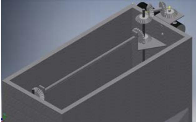
*Figure 1. Proposed Solution: bevel gears and rod. This solution was not chosen because of the many moving parts required. The torque requirements for a motor would also be high compared to other solutions. The parts involved in making this solution are also very expensive.*
