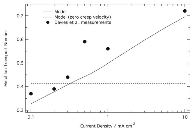
**Figure 8.** Comparison of model predictions with measurements of  $\text{Xe}^{125}$  marker positions for anodizing in 3% aqueous ammonium citrate solution.<sup>39</sup> Both experimental data and model predictions correspond to an oxide thickness of 145 nm. The model parameters were the same as those used to calculate the solid line in Fig. 5. The solid curve includes the effect of oxide flow, while the dashed line assumes that the oxide velocity is zero.
