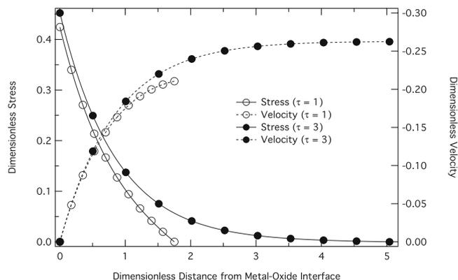
**Figure 2.** Calculated dimensionless stress and creep velocity profiles in anodic films for two selected times during anodizing at 3 mA/cm<sup>2</sup>.
