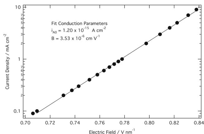
**Figure 6.** Dependence of anodizing current density on the calculated average electric field in the oxide film. The markers are model results, and the solid line is a linear regression fit. At a given current density, film thicknesses of 50–450 nm yielded the same electric field to three significant digits. The model parameters were the same as those used to calculate the solid line in Fig. 5.
