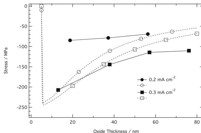
**Figure 4.** Comparison of model calculations with measurements of stress variation with anodic film thickness (compressive regime). Solid markers are stress measurements after interruption of anodizing at current densities of 0.2, 0.3, and 0.4 mA/cm<sup>2</sup>.<sup>21</sup> The dashed curves and open markers are model calculations. Model parameters: Viscosity  $\eta = 1 \times 10^{12}$  Pa s and minimum interfacial stress  $\sigma_{xx}^{\min} = -500$  MPa.
