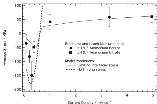
**Figure 5.** Dependence of stress in anodic films on current density. Markers are stress measurements after current interruptions, and vertical bars represent the variability of stress with oxide thickness over a range to 15–300 nm.<sup>9</sup> Curves are model calculations with no limiting interfacial stress (dashed line) and with  $\sigma_{xx}^{\min} = -500$  MPa and  $\sigma_{xx}^{\max} = 200$  MPa (solid line). The viscosity was  $1 \times 10^{12}$  Pa s.
