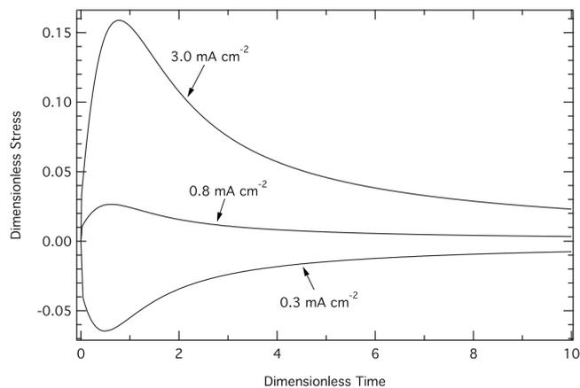
**Figure 1.** Variation in dimensionless stress with dimensionless time at three selected current densities. The velocity was set to zero at the metal–film interface.
