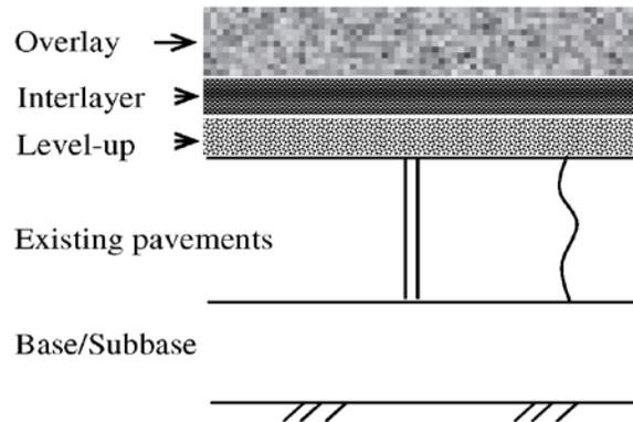
Fig. 1. Sketch of a HMA overlay system.
