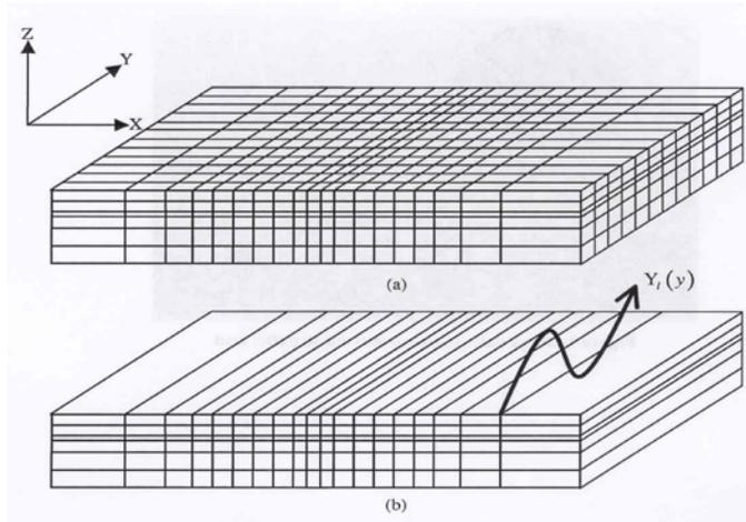
Fig. 3. A pavement section, where X is the direction of traffic: (a) 3D Finite Element Analysis; (b) Finite Element Analysis in the X-Z Direction and a Modal analysis in the Y direction.
