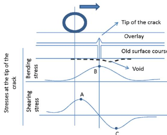
Fig. 2. Shear and bending stress induced at a crack caused by a moving wheel load (after Lytton, 1989).
