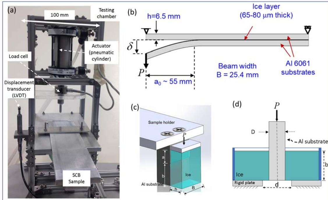
Fig. 2 (a) Developed universal testing setup. (b) Single cantilever beam testing configuration. (c) Direct shear-testing configuration. (d) Push-out testing configuration.
