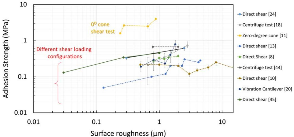
**Fig. 1 Summary of reported ice adhesion strength for an ice/aluminum interface using different experimental loading configuration. A full order of magnitude difference can be observed between 0° cone angle shear test and other testing configuration.**
