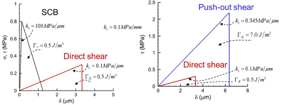
**Fig. 7** The experimentally guided and numerically fitted bilinear traction-separation correlations for (a) normal and shear cohesive relations, and (b) shear cohesive relationship for different shear configurations.
