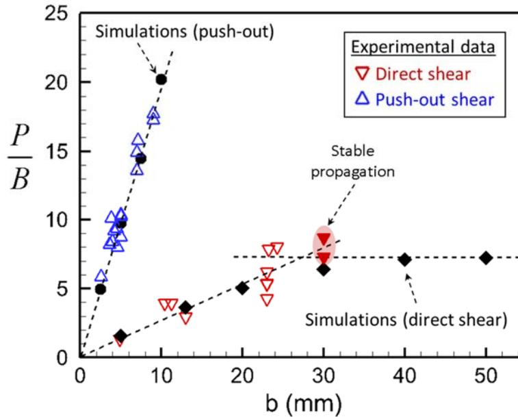
**Fig. 6 Summary of the experimental and numerical results for the interfacial normalized decohesion force (by the sample width) vs. the shear ice length for both the direct shear and push-out shear tests. The initial slope of the curve is the interfacial shear strength of the ice-solid interface.**
