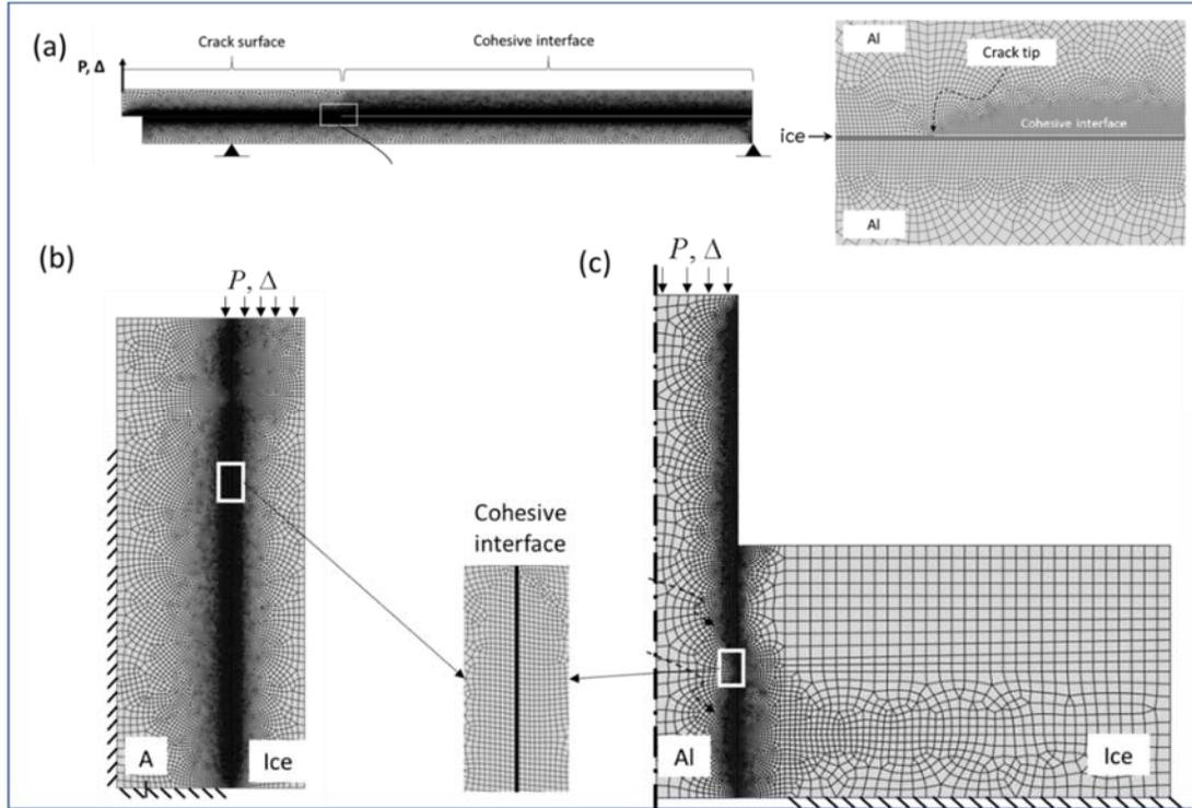
**Fig. 3** Finite element models for (a) SCB(plain strain) , (b) direct shear (plane strain) and (d) push-out shear (axisymmetric) testing geometries.
