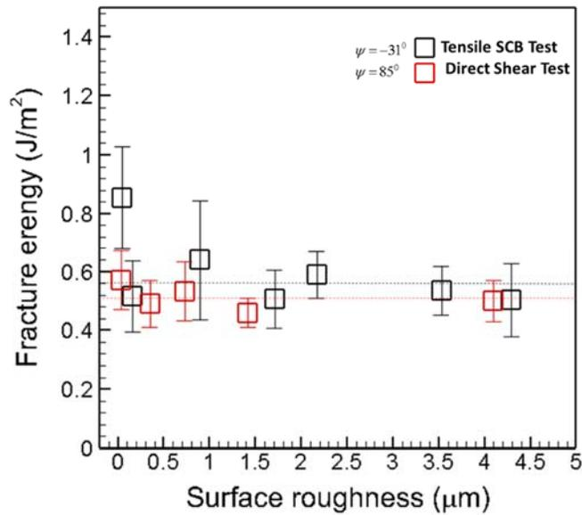
**Fig. 5 Summary for the experimental measurements for the interfacial fracture energy as a function of the surface RMS roughness at  $-17^\circ\text{C}$ . SCB samples are for  $a=55\text{ mm}$  crack, and direct shear samples have  $b=13\text{ mm}$  ligament and  $B=20\text{ mm}$  width.**
