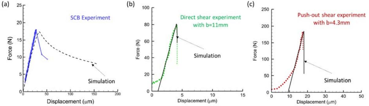
**Fig. 8** Comparison between the experimental measured and FEA simulated force-displacement curves obtained for the different configurations. (a) Single cantilever beam test. (b) Direct shear test. (c) Push-out test.
