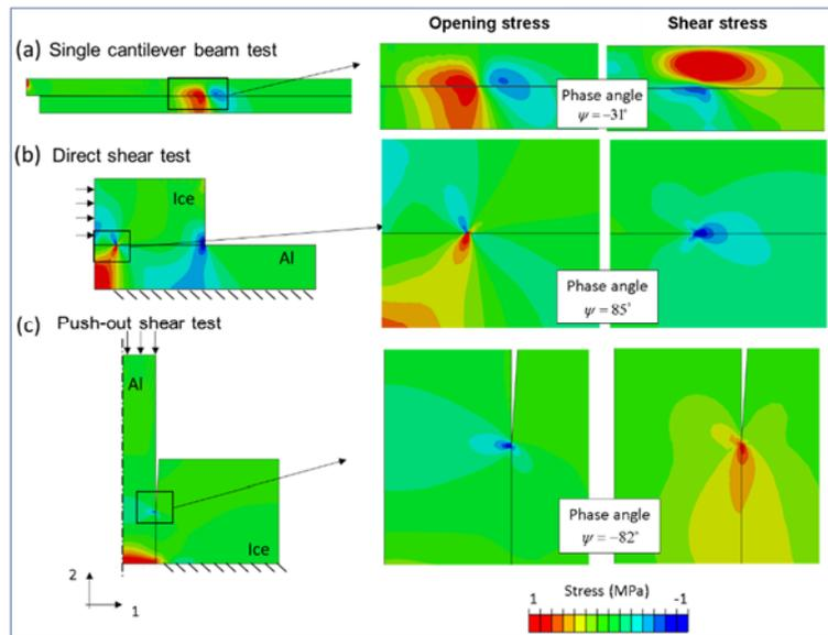
Fig. 4 FEM results for opening and shear stress fields near the crack tip for all examined configurations.
