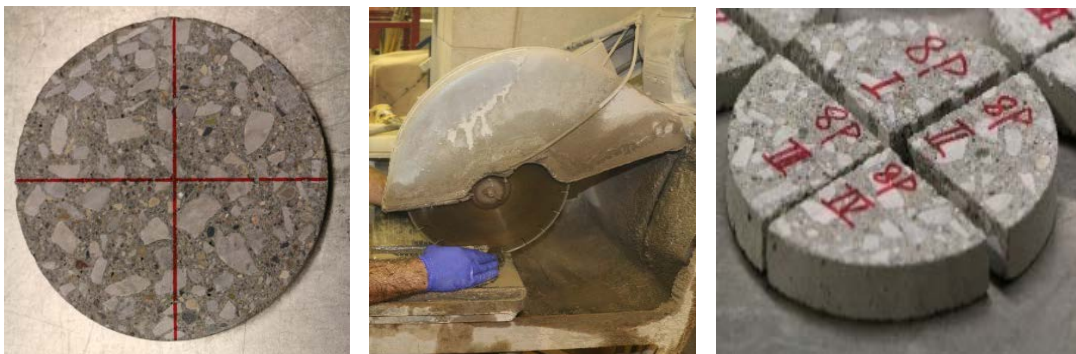
Figure 1. Preparation of PCC substrates in the laboratory.
