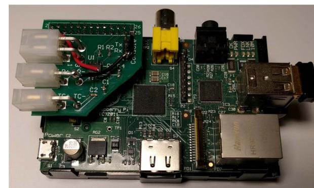
Figure 2: The assembled board mounted to the Raspberry Pi.
