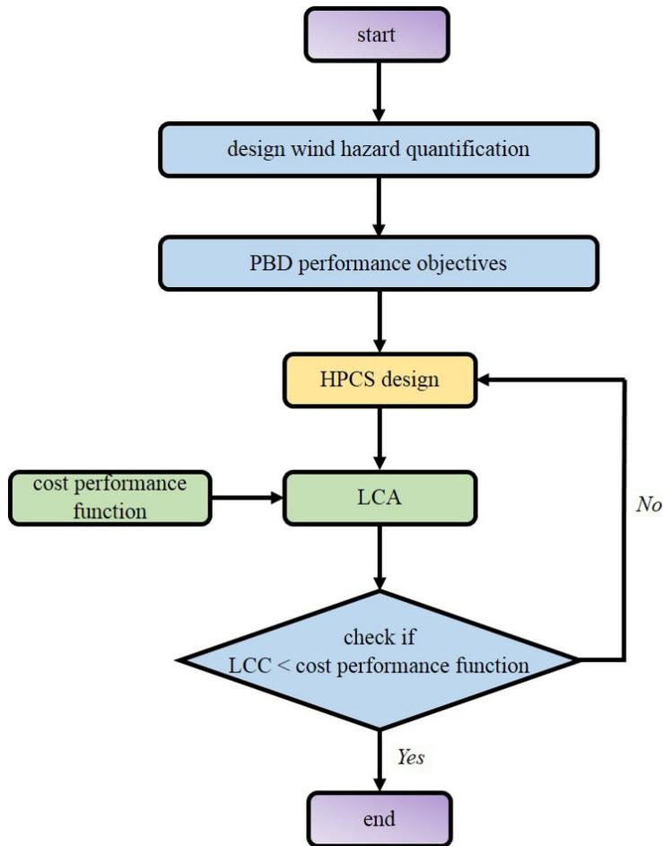
Figure 1: Proposed PBD procedure for HPCS used in wind hazard mitigation
