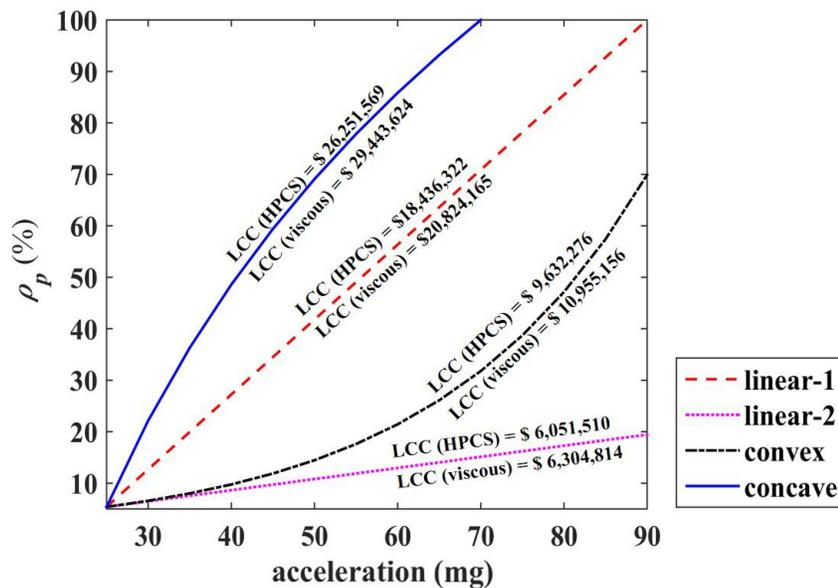
Figure 7: Assumed relationships between  $\rho_p$  and  $\max(\ddot{x})$  and associated LCC values
