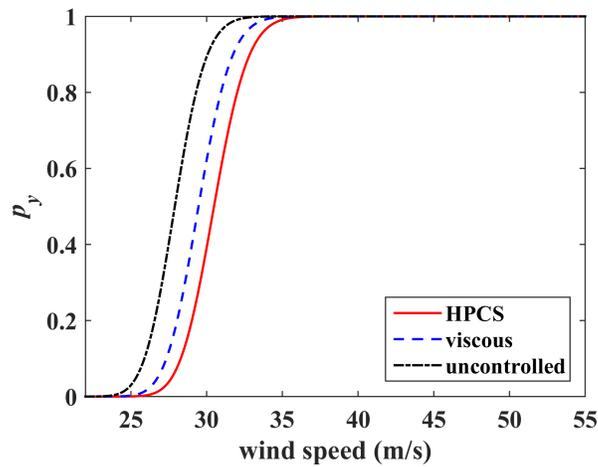
Figure 5: Estimated probability  $p_y$  for extreme acceleration level
