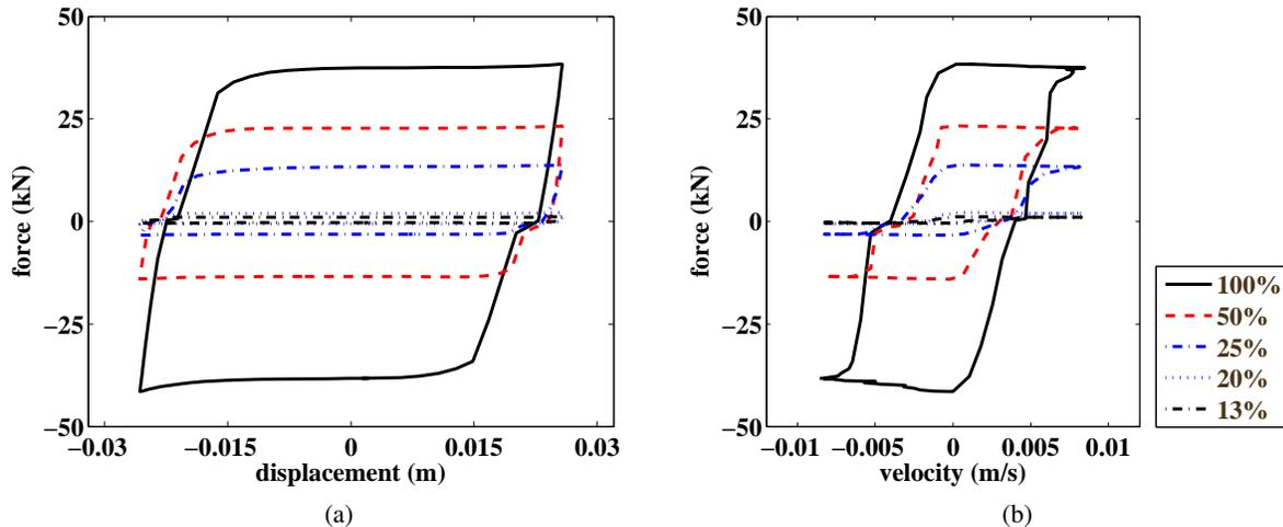
Figure 3: Modeled dynamics of the BRFD under various applied forces under a 0.05 Hz excitation of 25.4 mm (1 in) amplitude: (a) force-displacement; (b) force-velocity
