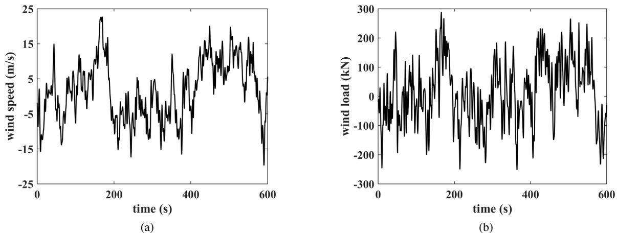
Figure 4: The extreme wind hazard level at 36<sup>th</sup> floor: (a) time series of wind speed  $V_{w,36}(t)$ ; and (b) time series of wind drag force  $P_{w,36}(t)$ .
