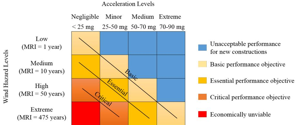
Figure 2: Performance-based matrix for wind excitations
