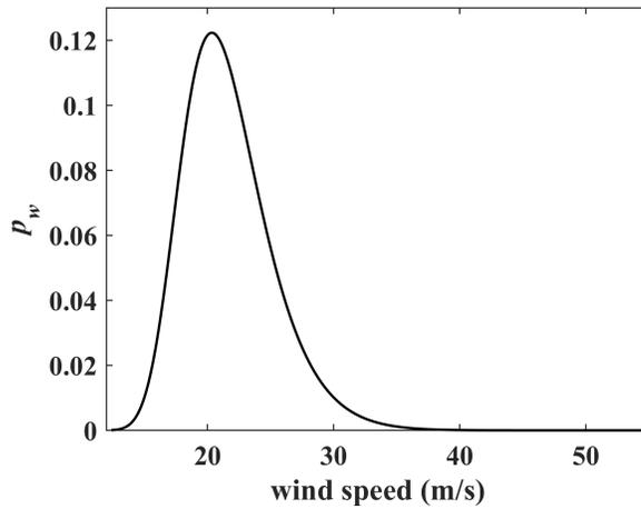
Figure 6: Wind speed hazard function  $p_w$  at height  $h = 130$  m
