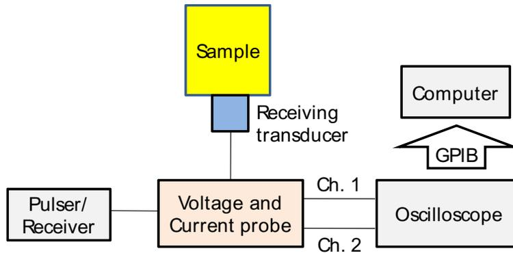
**FIGURE 1.** Schematic diagram for calibration of receiving transducer.
