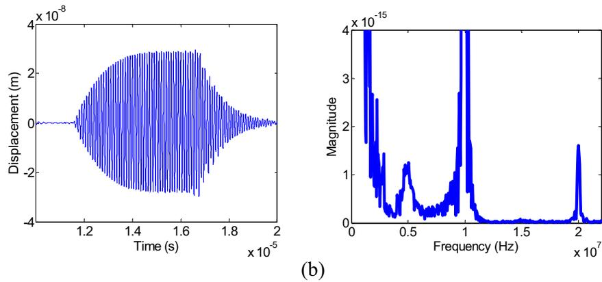
**FIGURE 6.** Harmonic generation measurement at position 2 with 0 dB input excitation: (b) Received waveform and Fourier spectrum after calibration.
