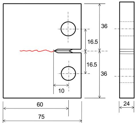
**FIGURE 3.** Configuration of CT specimen with fatigue crack (unit: mm).
