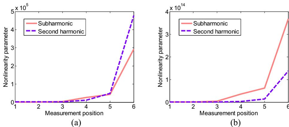
**FIGURE 7.** Variation of nonlinearity parameter as a function of measurement position: (a) Before calibration, (b) After calibration.
