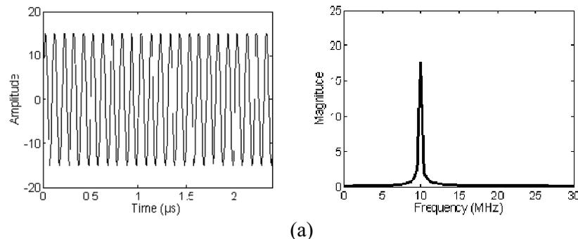
FIGURE 8. Simulation results for harmonic generation at a crack interface: (a) Input waveform and Power spectrum.
