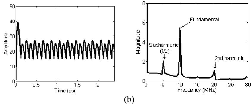
**FIGURE 8.** Simulation results for harmonic generation at a crack interface: (b) Output waveform and power spectrum.
