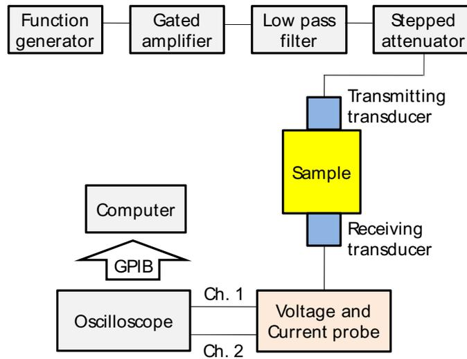
**FIGURE 2.** Schematic diagram for harmonic generation measurement.
