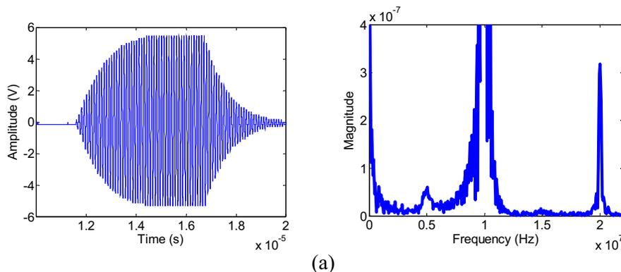
FIGURE 6. Harmonic generation measurement at position 2 with 0 dB input excitation: (a) Received waveform and Fourier spectrum before calibration.
