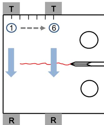
**FIGURE 4.** Harmonic generation measurements at six positions along the cracked interface.
