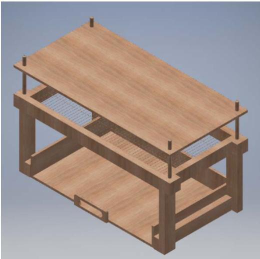
**Solution 1 Prototype: Foam Block Cutting Jig**
