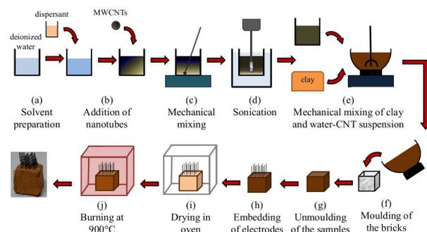
Fig. 1. Fabrication process of nanocomposite clay bricks.
