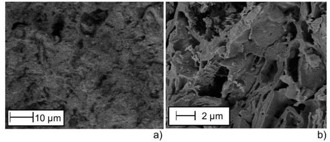
Fig. 2. SEM images of normal clay bricks after drying (a) and after burning at 900 °C (b)
