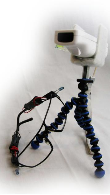
**FIGURE 3. WII REMOTE, TRIPOD MOUNT, AND TRACKABLE GLASSES**
