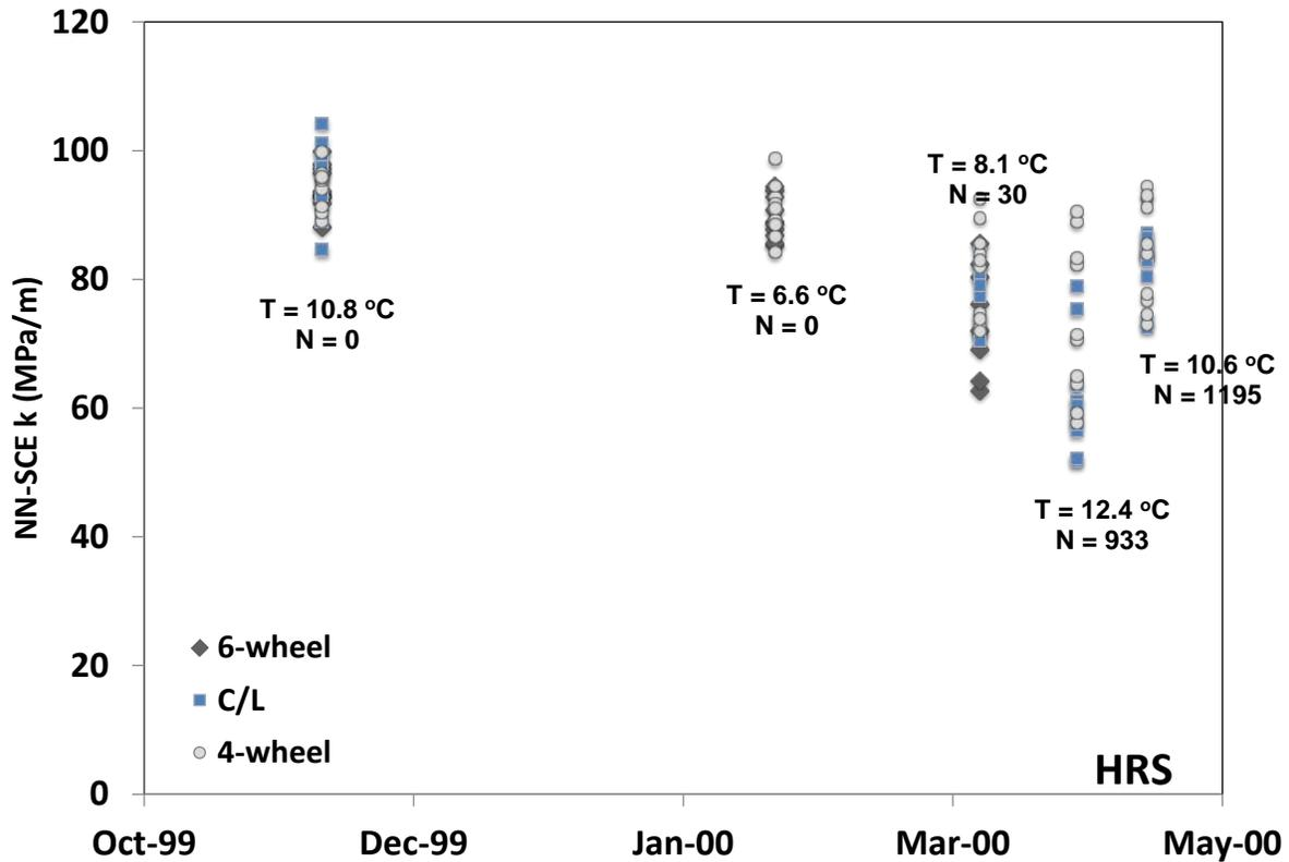
**Figure 13.** NN-SCE predicted k-values for HRS during traffic testing
