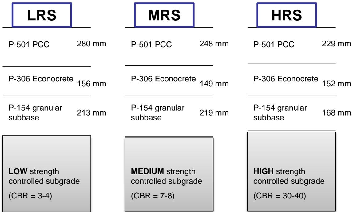
**Figure 9.** Schematic of NAPTF CC1 rigid pavement items cross-sections
