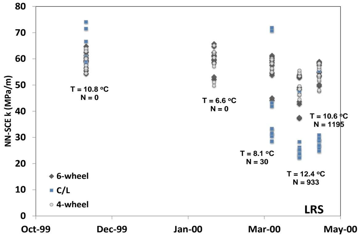
Figure 11. NN-SCE predicted k-values for LRS test section during traffic testing
