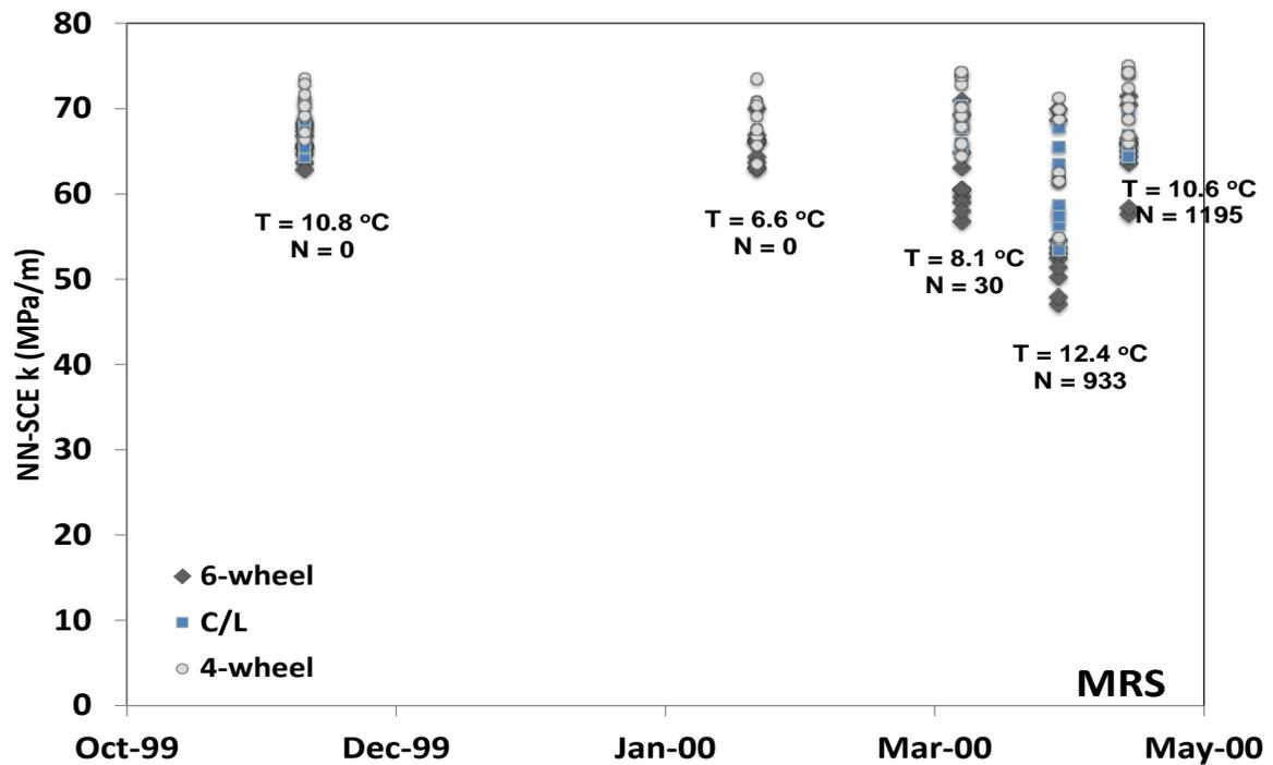
Figure 12. NN-SCE predicted k-values for MRS during traffic testing
