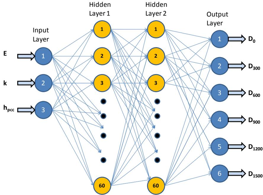
**Figure 5.** NN surrogate forward pavement response model architecture
