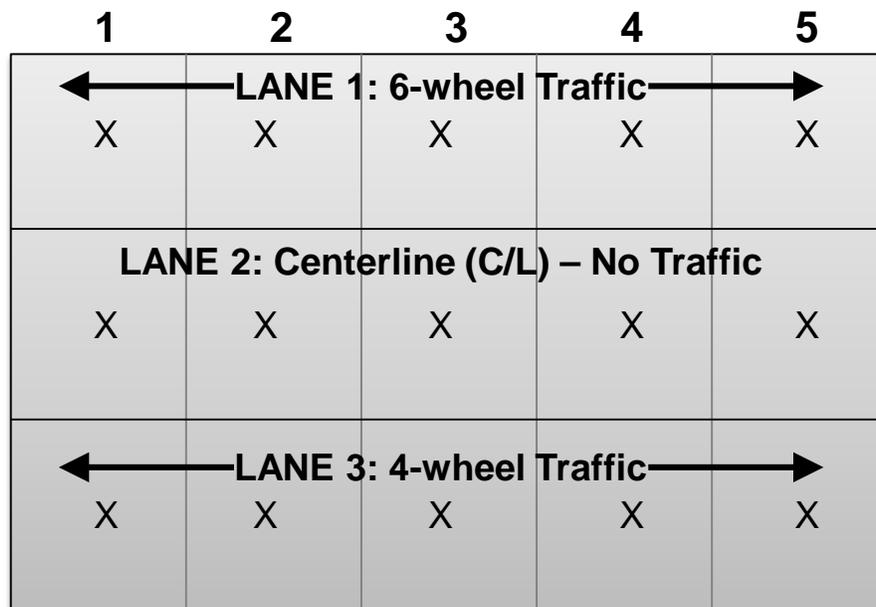
**Figure 10.** Schematic of NAPTF CC1 rigid pavement NDT slab center test locations
