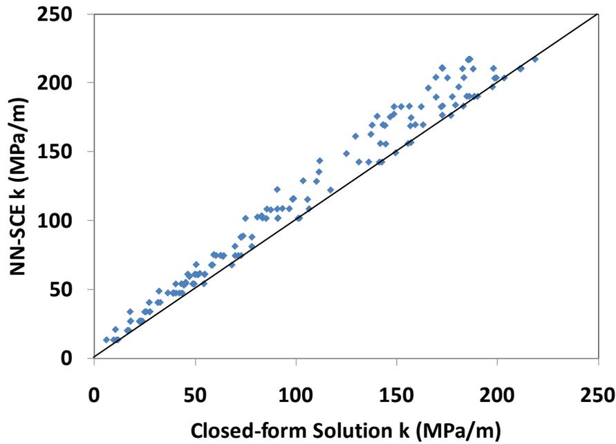
**Figure 8.** NN-SCE k predictions compared with closed-form solutions
