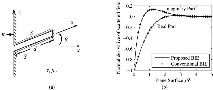
**FIGURE 2.** (a) Configuration of thin crack in a half-space conductor. Surface  $S^+$  and  $S^-$  are the upper and lower surfaces of the crack, respectively. (b) Normal derivative of scattered field on the plane surface for a perpendicular crack with depth  $d = 4\delta$ . Values are normalized by the surface impedance for the half-space conductor. Numerical results calculated from proposed (solid line) and conventional (plus sign) BIE are shown.
