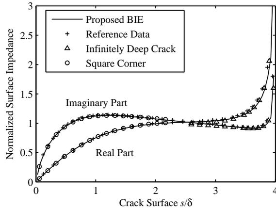
**FIGURE 3.** Normalized surface impedance on the crack surface for a perpendicular crack with depth  $d = 4 \times \delta$ . The results (solid line) are calculated using the proposed BIE. Kahn's results [11] for the ideal crack (plus sign) are plotted. The analytical solution for the infinitely deep crack (triangle) and square corner (circle) are also shown for comparison.
