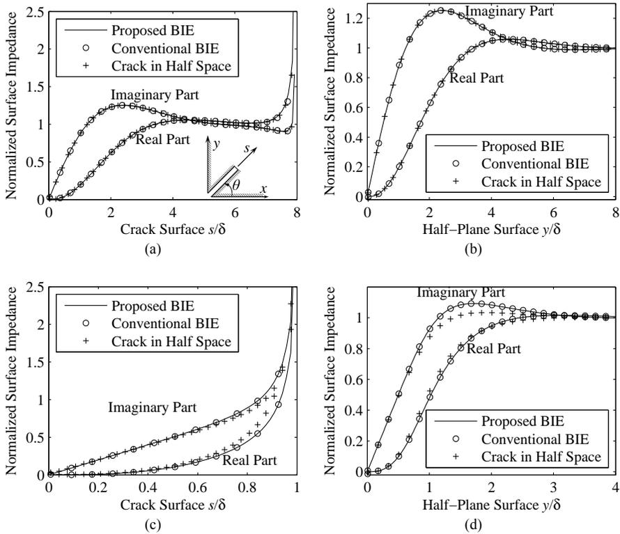
**FIGURE 6.** Normalized surface impedance for cases with  $d = 8\delta, \theta = 45^\circ$  (a, b) and  $d = \delta, \theta = 45^\circ$  (c, d). Numerical results from proposed (solid line) and conventional (circle) BIEs are shown. The results for the surface crack in a half-space conductor with same inclination angle (plus sign) are also plotted.
