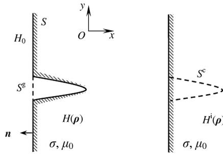
**FIGURE 1.** Schematic configuration of the surface crack problems with uniform applied field  $H_0$ .  $H^i$  is the incident magnetic field in the absence of the crack.  $S^c$  and  $S^g$  represent crack surface and “gap” surface, respectively.
