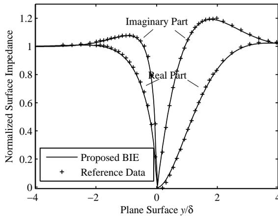
**FIGURE 5.** Comparison of result from Kahn (plus sign) [11] and that calculated from the proposed BIE (solid line) for the normalized surface impedance on the plane surface:  $d = 3\delta$ , and  $\theta = 30^\circ$ .
