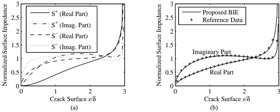
**FIGURE 4.** Normalized surface impedance over the crack surface for a crack with  $d = 3\delta$ , and  $\theta = 30^\circ$ . The results on both sides of the crack (a) and the average value of them (b) are plotted. Also Kahn's results [11] for the ideal crack (plus sign) are shown in (b).
